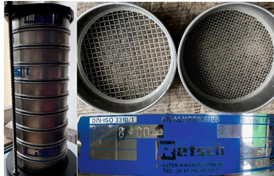
Figure 6: Sieve cascade (left) with sieve of different mesh sizes (top), sieve designation (bottom)
