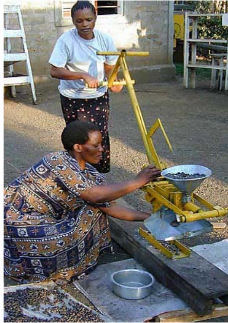
Figure 4.4 Simple Home Based Jatropha Oil Press.
