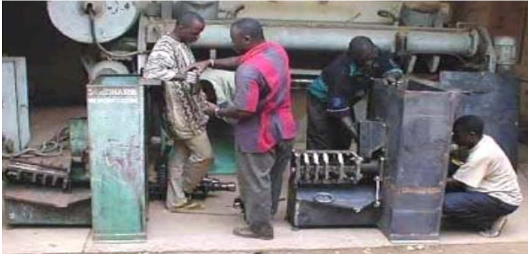
Figure 4.5 Locally manufactured Industrial Jatropha oil Press.
