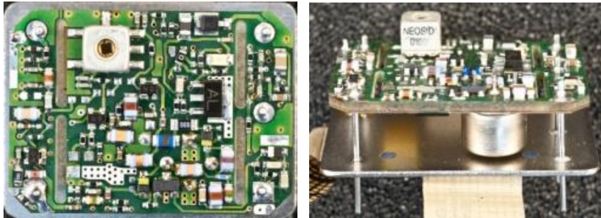
Figure 7-9: shows the prototype 5 th overtone 125 MHz crystal (crystal resonator unloaded Q=90,000)[13]
