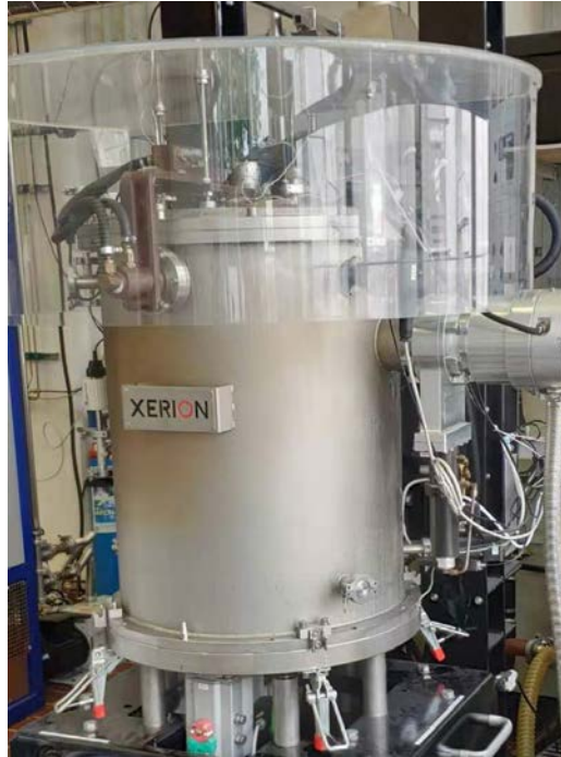
Fig. 4.2-3. Vacuum sintering furnace
