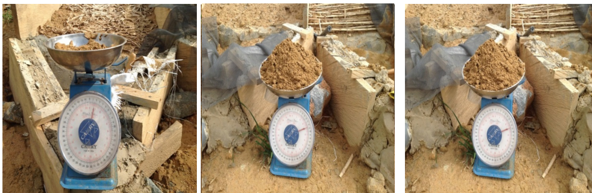
Figure 2. 7: First sediment yield collection and weighing after installation; left (control) = 36.8 kg; middle (YM) = 0.8 kg; right (EM) = 3.5 kg.
