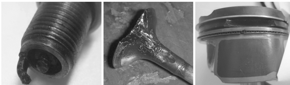
Figure 2.5: Damaged cylinder parts due to super knock [32].
