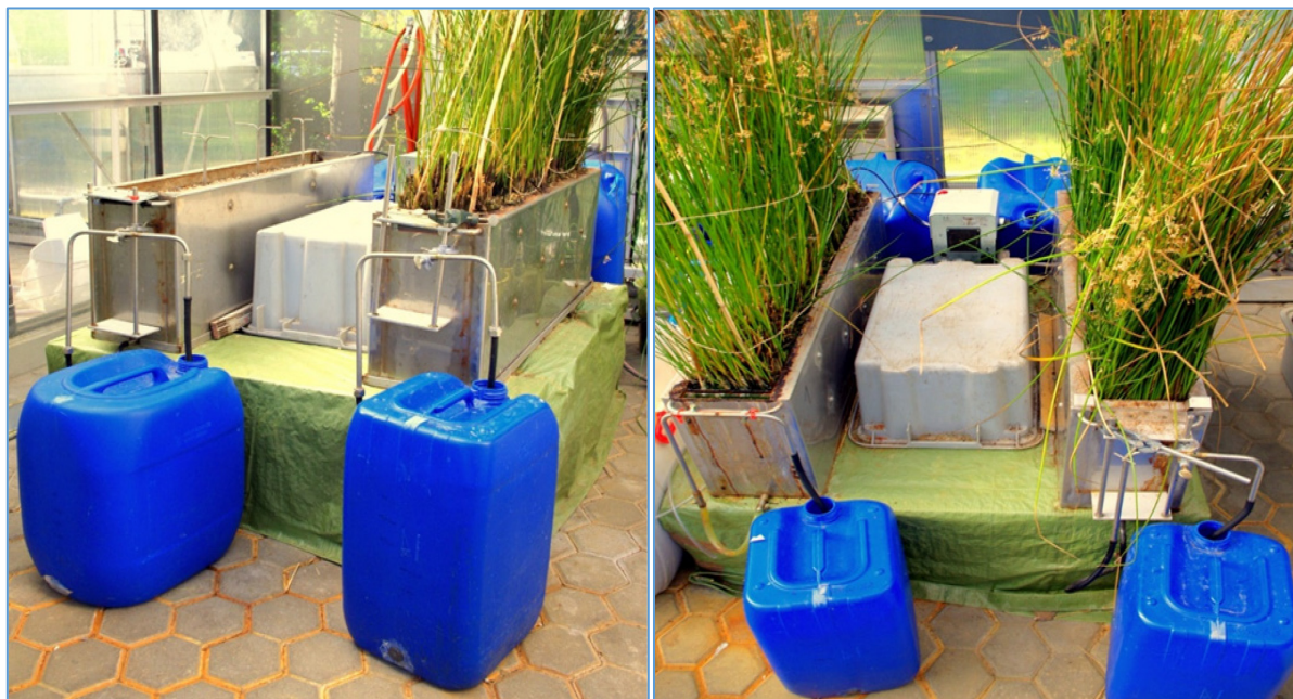
Figure 2. 2- Laboratory scale experimental set up in green house planted with Juncus effuses
