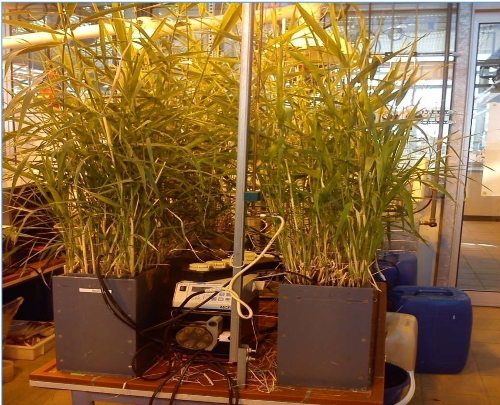
Figure 2. 6- Laboratory scale experimental set up in Phytotechnicum planted with Phragmites australis
