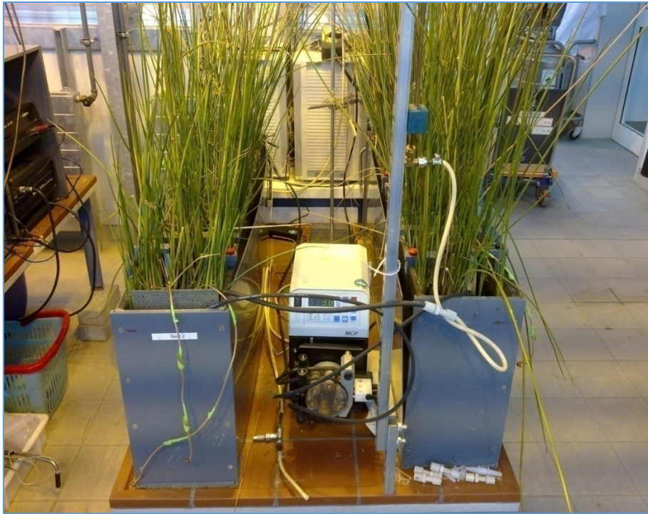
Figure 2. 4- Laboratory scale experimental set up in Phytotechnicum planted with Juncus effuses
