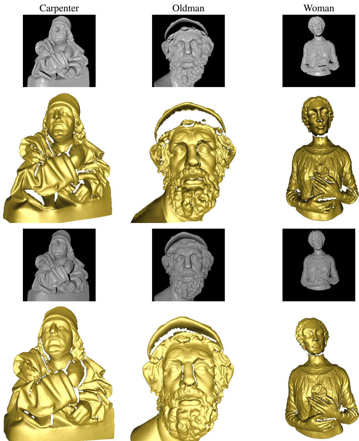
Figure 4-7: First row: input specular images with directional light [73]. Second row: our 3D output using DLPS. Third row: input images with pointwise light. Last row: our 3D output with PLPS. Images produced by directional light are imposed by more specularly and shadows in comparison with images with pointwise light. These shadow parts lead to losing some reconstructed area.
