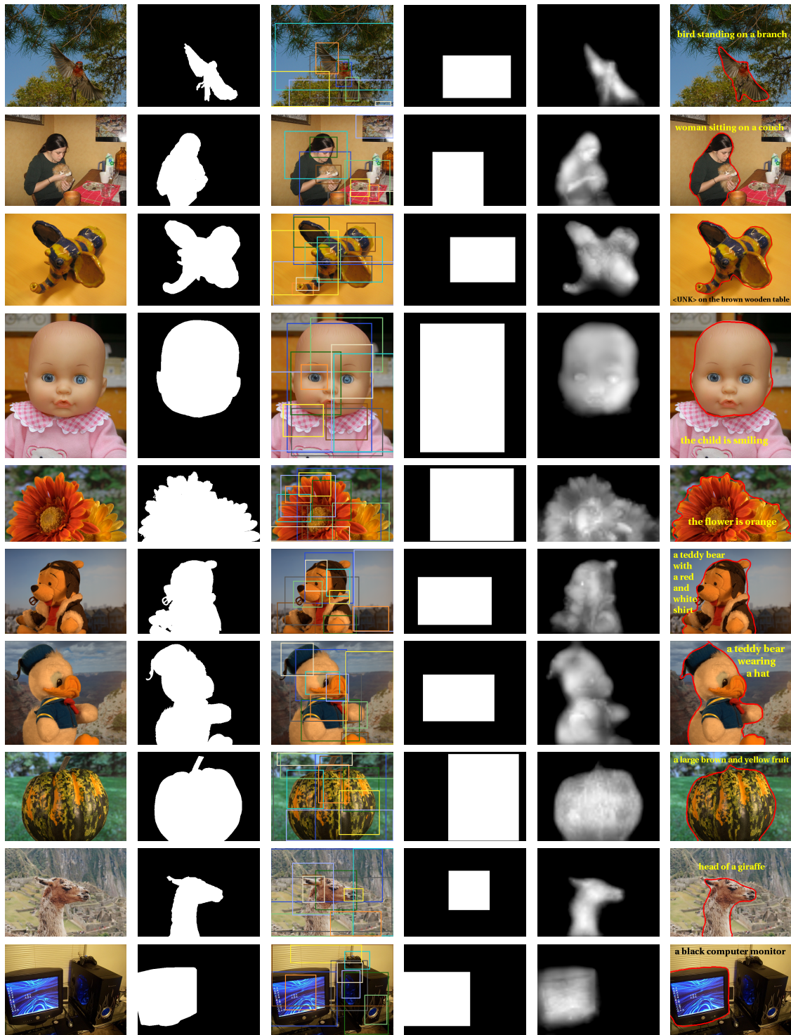
Figure 3-14: Operating progress of our proposed hybrid model, from left to right: input images obtained from [165], [136], [13], [183] or [62], UIR ground truths, dense captioning bounding boxes, best match bounding boxes, the probability maps of our interactive segmentation module and the final outputs of our model including highlighted UIR and its description.
