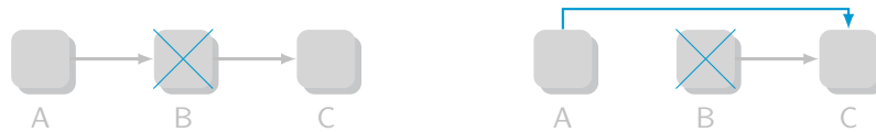
(a) Thread 1 started to remove element B (b) Thread 1 removed element B completely by setting a marker.
