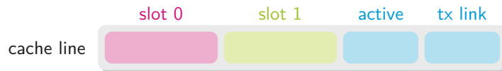
Figure 4.20: Cache line layout for MCL-TXID. Meta data does not only contain an active bit, but also a link to the most recent transaction which modified the cache line.
