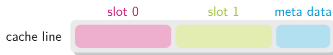
Figure 4.3: Cache line layout. Two slots store data and the remaining part is for meta data.
