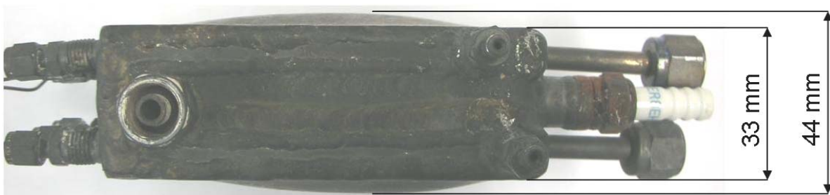
Figure 9 Bulge of reformer reactor walls after deformation → possible bypass
