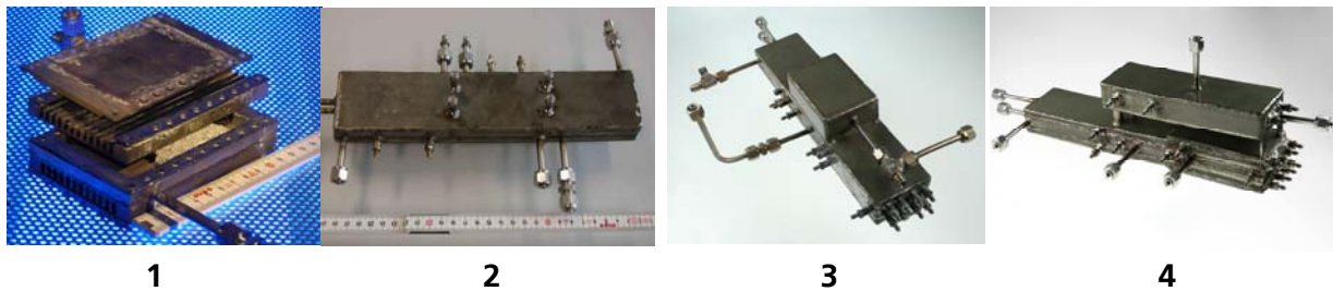
Figure 24: Progress in reactor design (left to right): reformer-burner-sandwich only (1), with evaporator and superheater (2), with additional MTS (3), with HTS and LTS (4)
