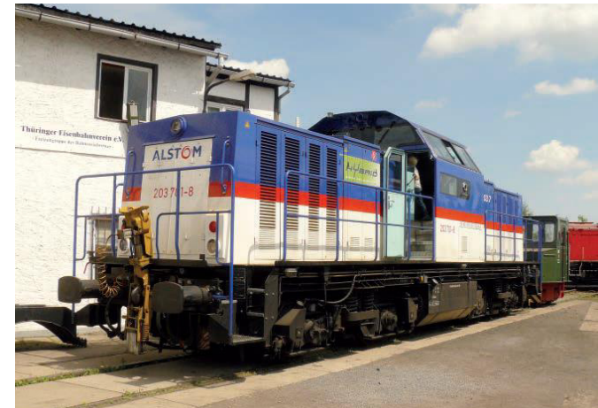
Hybridrangierlokomotive (BR203H von Alstom) 2
