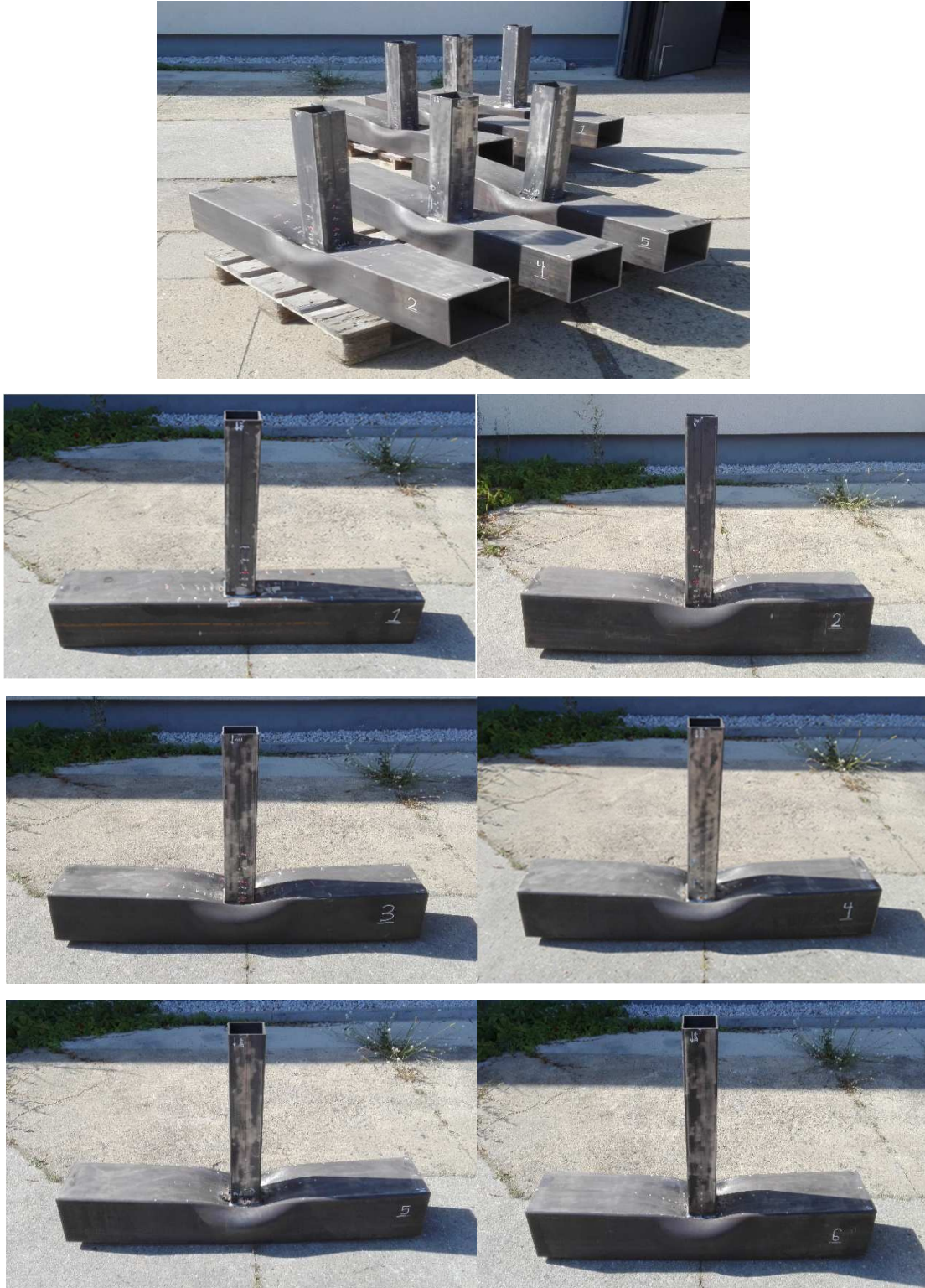
Figure 4.31: Failure modes joint 1 to 6.
