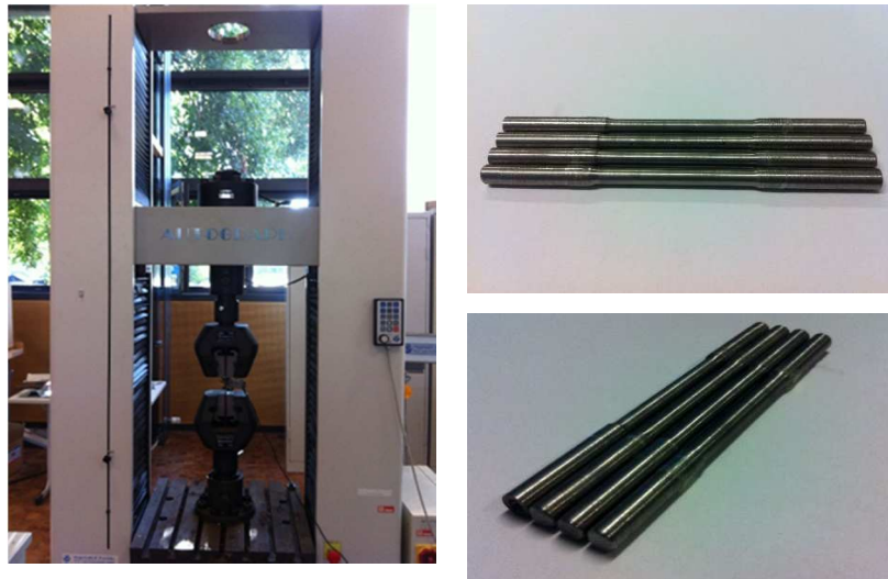
Figure 4.1: Universal testing machine UTM (left) and material testing specimen (right).
