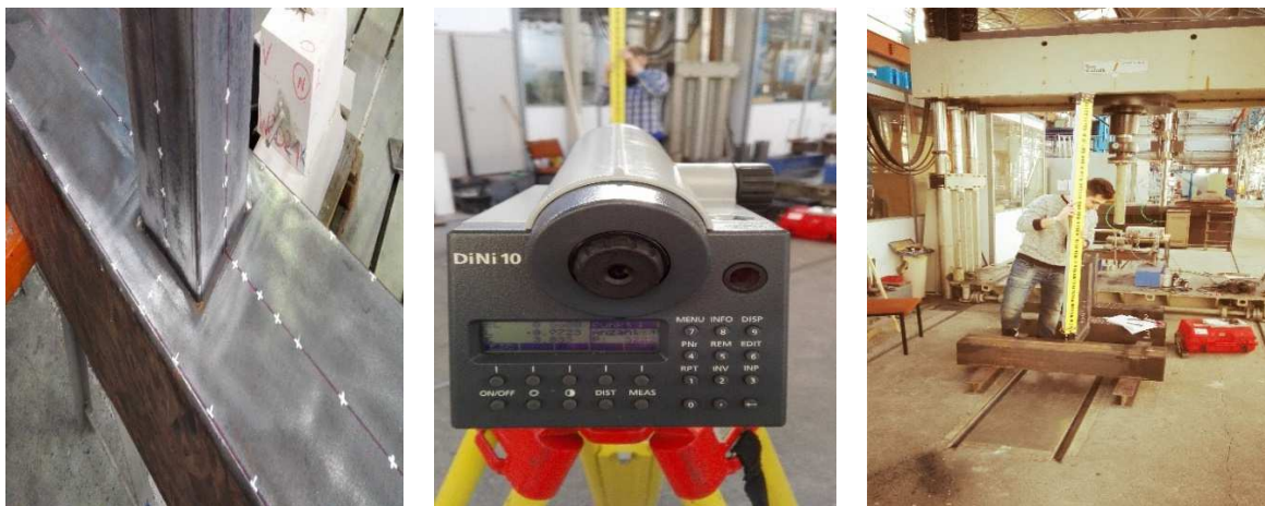
Figure 9.1: Measuring the initial geometry by using surveying camera.
