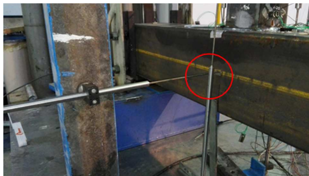
Figure 4.22: First test, failure in the displacement transducers 5 and 8.
