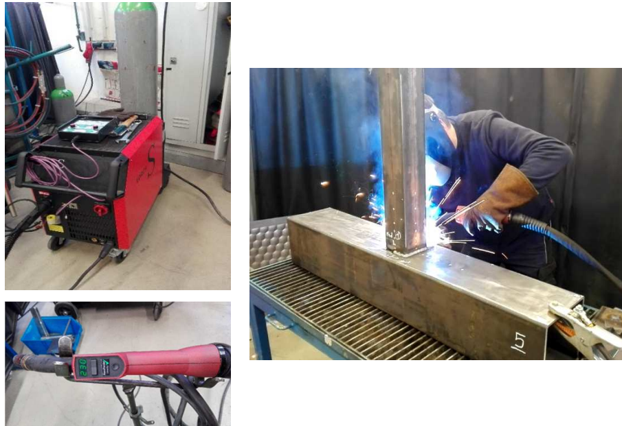
Figure 4.6: Welding procedure and the welding machine.
