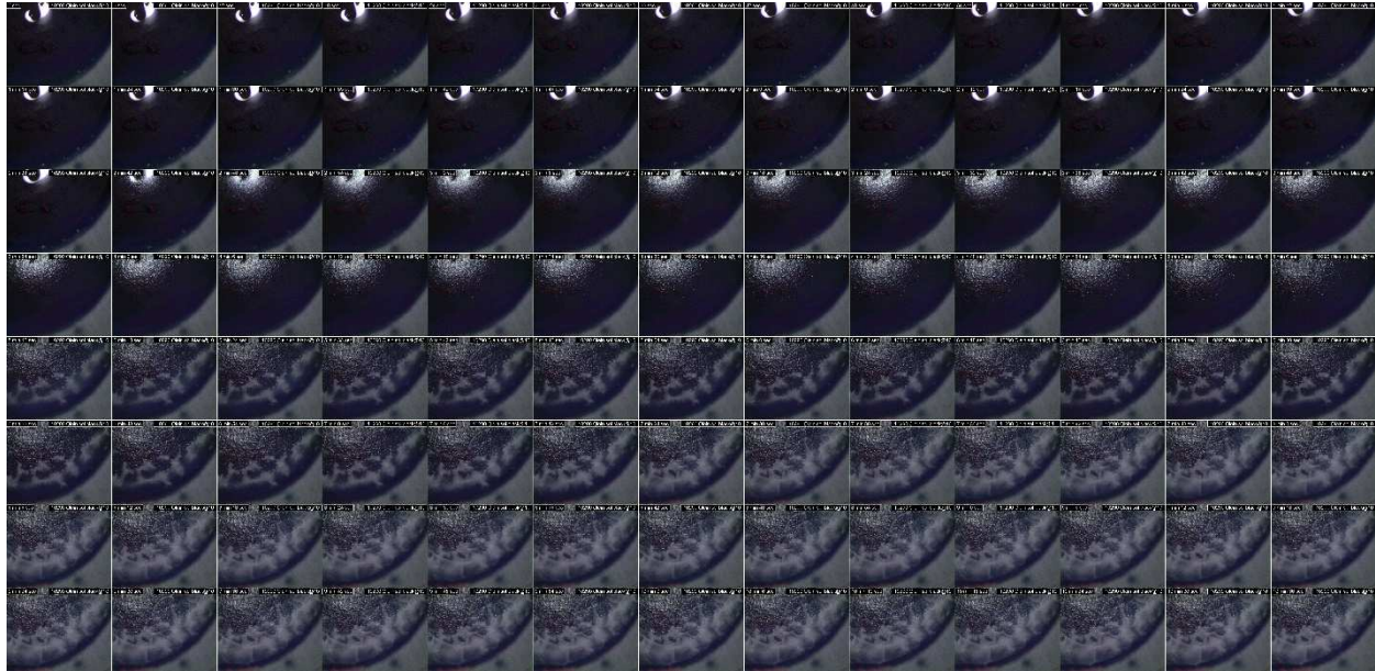
FIGURE 1-7: PHASE BEHAVIOR OF ENRICHED CRYSTAL FRACTION OF HIGH OLEIC SUNFLOWER OIL @ 10 KMIN-1 , 50°C TO - 60°C IN AN OXIDIZED BLACK COPPER CRUCIBLE 27
