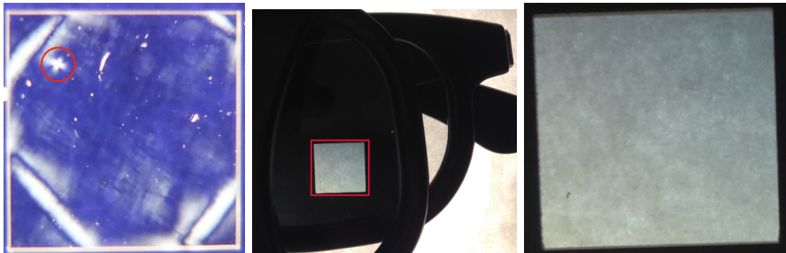
Figure 5.3: Picture of the diamond [106] (left) and sapphire (middle, right) through linear polarized films of the cinema goggles.
