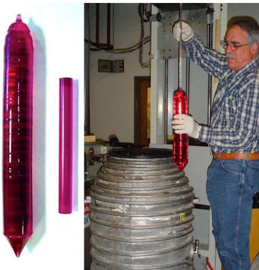
Figure 5.2: A Czochralski-grown synthetic ruby crystal is shown alongside a fabricated piece (left), and during removal from the growth station (right). Photos by Jennifer Stone-Sundberg [101].
