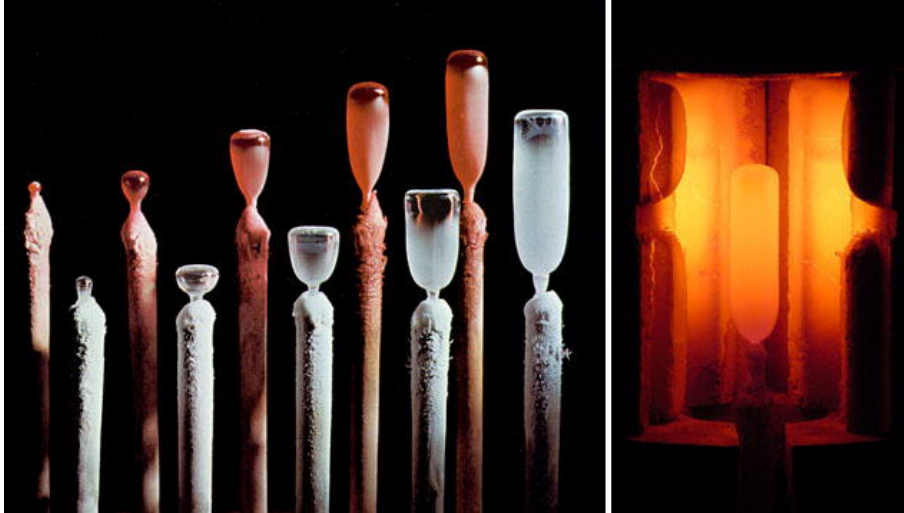
Figure 5.1: These photos show flame-fusion synthetic sapphire crystals, as-grown (left) and during growth in the furnace (right). Courtesy of Hrand Djvahirdjian, SA [101].
