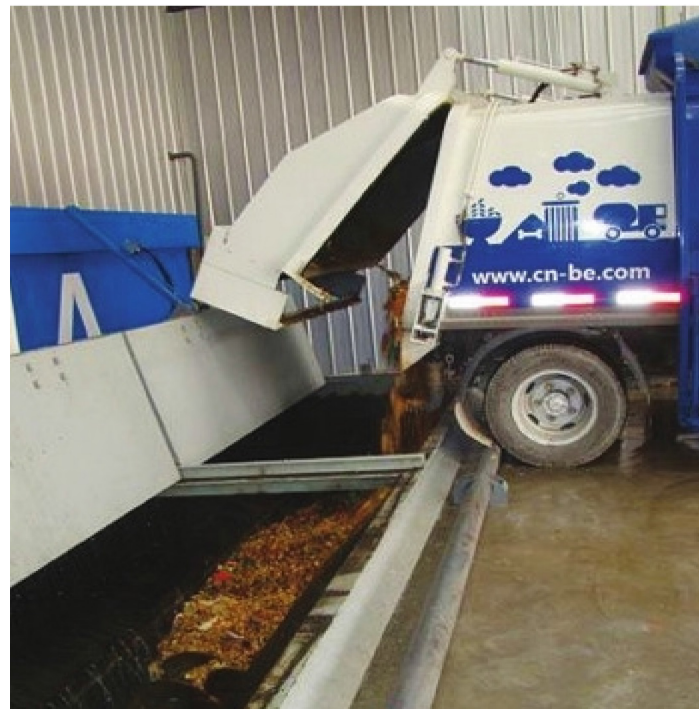
Figure 5-1: Waste Discharging in semi-percolator
