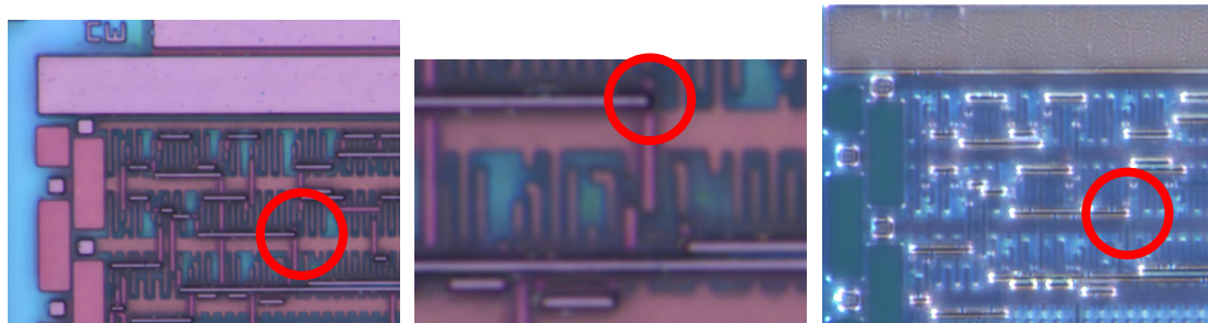
(a) Top view photograph of vertical metal2 and vias to horizontal metal3. In the red marked area a MIM structure is built-in (200x magnification). (b) Zoom in of Figure 72a (500x magnification). (c) Top view of 72a in dark field illumination.
