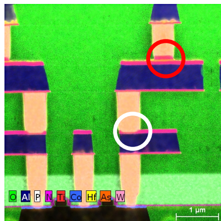
(b) EDX photograph of 73a. Different materials are marked in different colors. The difference between a via with a connection between two metal layers and the via including the isolation is clearly visible.
