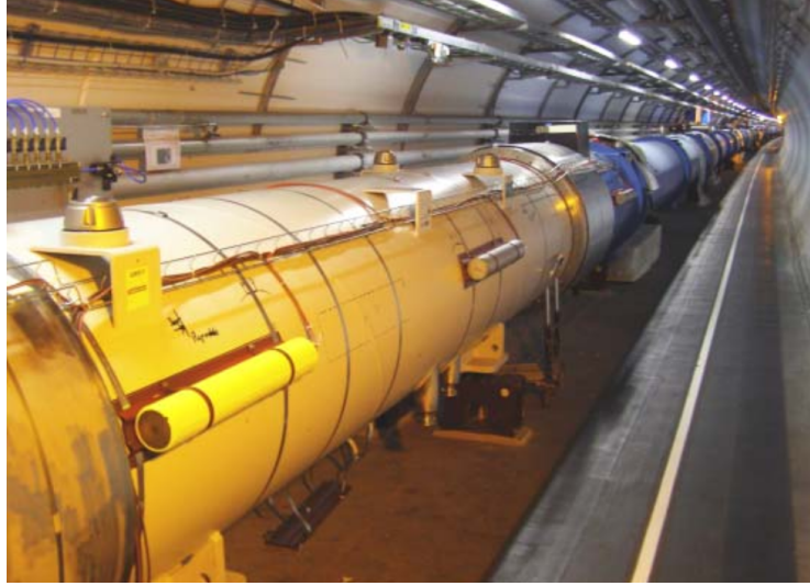
Figure 11: Ionization chambers in the little yellow cylinders and installed outside of a dipole magnet (taken from Reference [18]).
