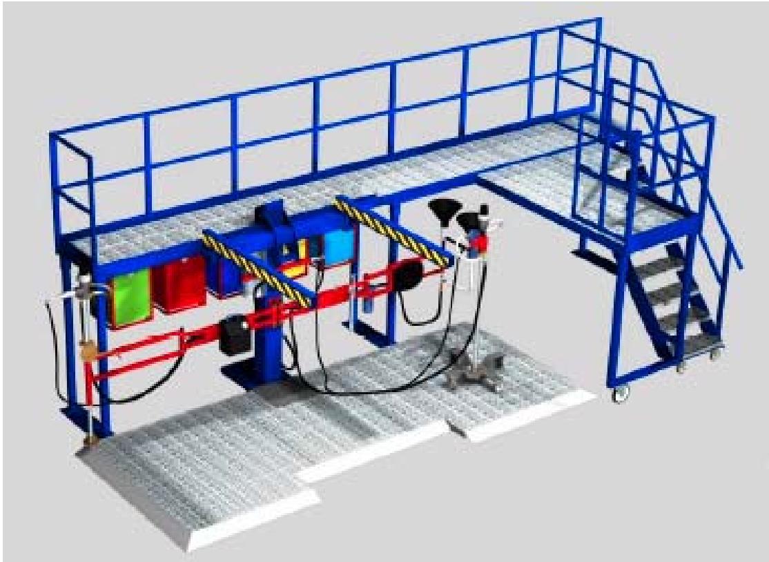
Figure C.2 De-pollution Rig with a Capacity of 50 ELV/day
