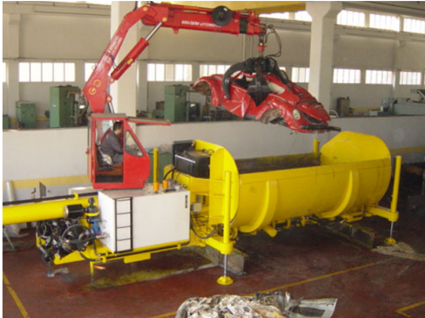
Figure C.10 Car Baler to Compact ELV in Dismantling Centres
