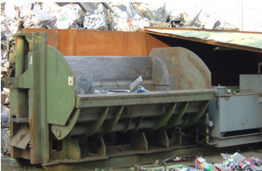
Figure C.11 Car Baler to Compact ELV in Dismantling Centres.
