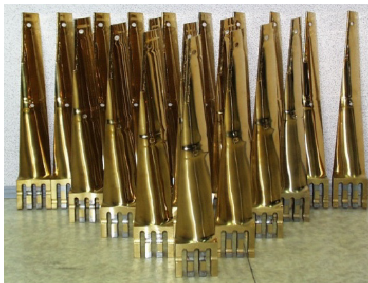
Figure 3. Industrial issue turbine blades with "slippery" coating.
