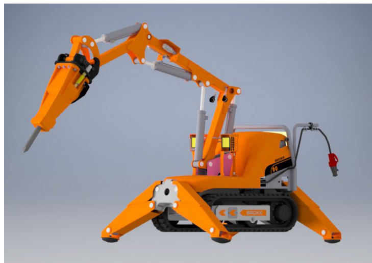
Fig. 2: Geometrical (CAD) model of the existing demolition robot
