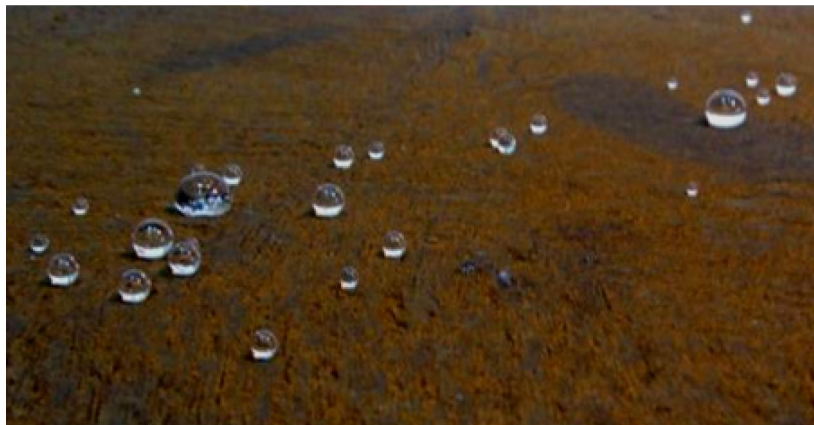
Figure 1. Drops of water on the metal surface after SAW technology.
