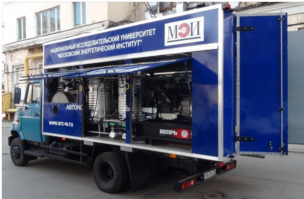
Figure 2. Mobile unit using to treat pipeline systems.
