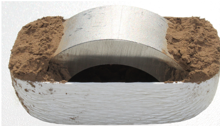
Figure 4.6.: Test specimen arrangement in half ceramic shell
