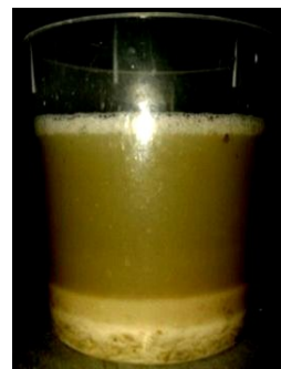
Picture 5-5: Hydrolysate after addition of hydrolysate from another anaerobic digester
