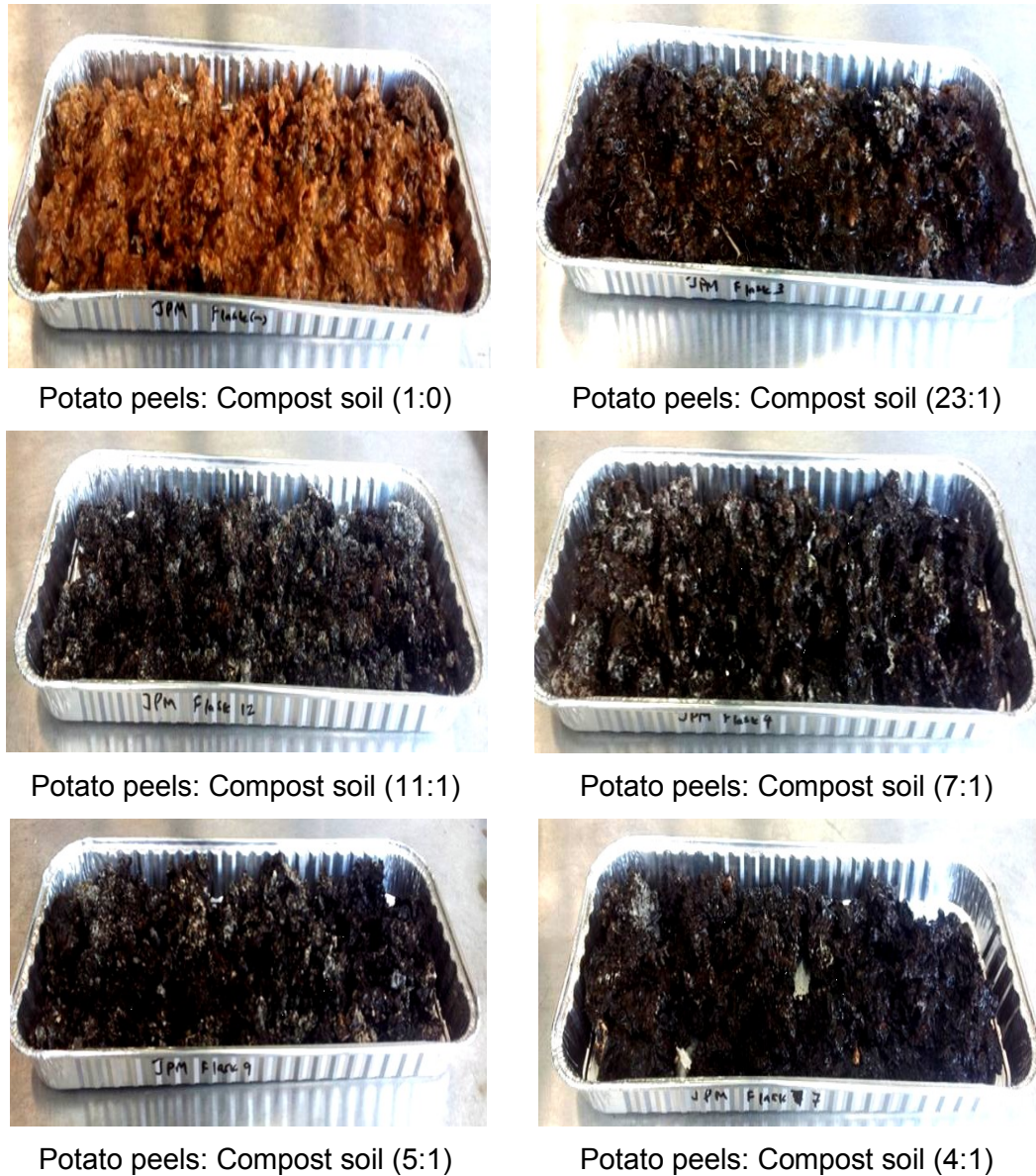
Picture 5-2: Attributes of compost from composting of air-dried potato peels
