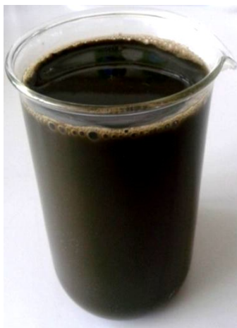
Picture 6-3: Digestate from Methanation reactor digesting contaminated potato peels
