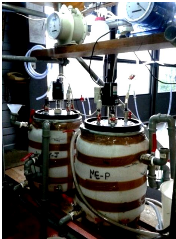
Picture 5-3: Set-up of two-phase CSTR anaerobic digestion system
