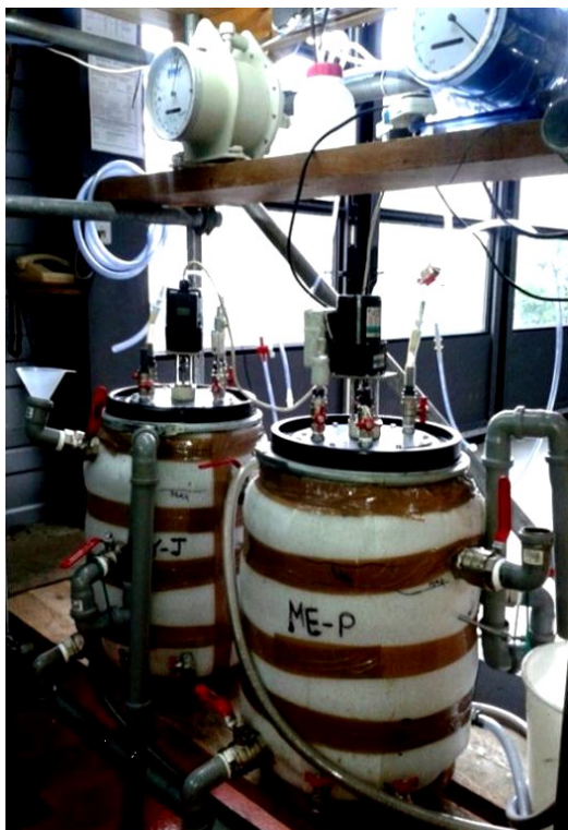
CSTR -front view with gas meters
