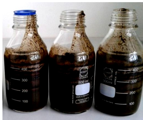
Picture 6-6: Lime conditioning of digestate
