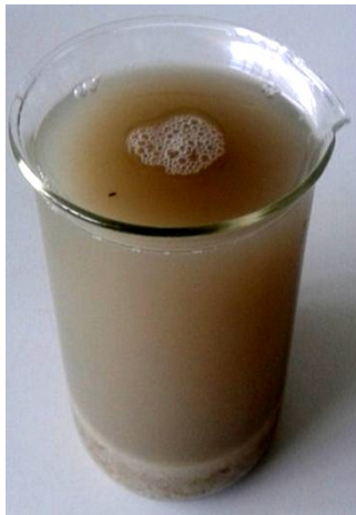
Picture 6-2: Digestate from hydrolysis reactor digesting contaminated potato peels
