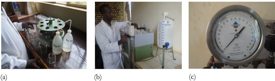
Figure 19: apparatus for determining soil aggregate stability and water holding capacity.
