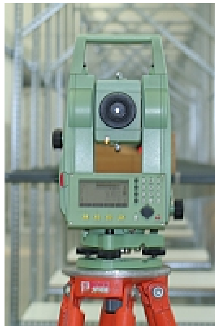
(a) Theodolite to survey the pipe test section.
