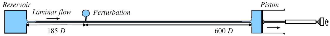
Figure 2.7: Schematic setup of the pipe flow facility for reverse transition investigations. Reprinted with permission from [J. Peixinho and T. Mullin, Physical Review Letters , 96(9):094501, 2006.
