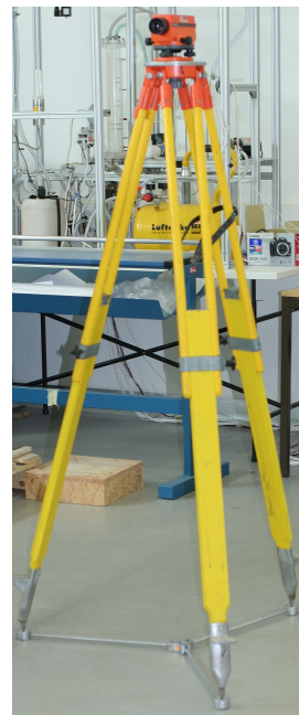
(b) Surveying level with tripod.
