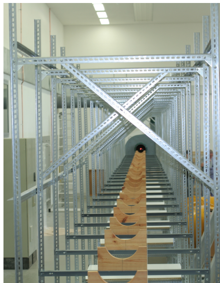
(b) CoLaPipe setup without pipe segments during surveying procedure with the blower unit at the end. The blower unit serves as connection and is therefore the initial point.
