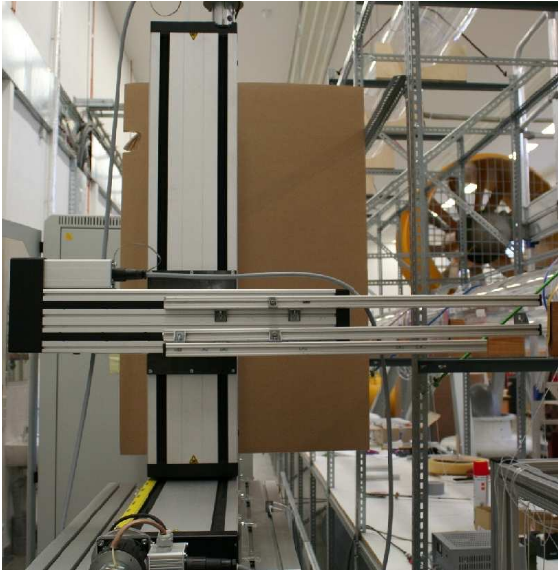
Figure 5.7: Traverse mechanism with independently moving components.
