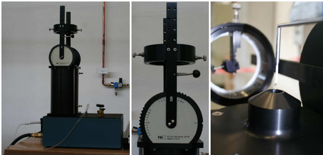
(a) Ex-situ calibration unit with air supply. (b) Variable angle adjustment. (c) Calibration unit contraction with probe to be calibrated.
