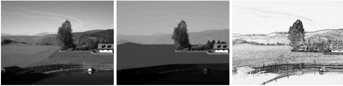
Figure 5.3: Different understanding of edges in an image; from left to right: original image, interesting regions, edges based on gradient detection
