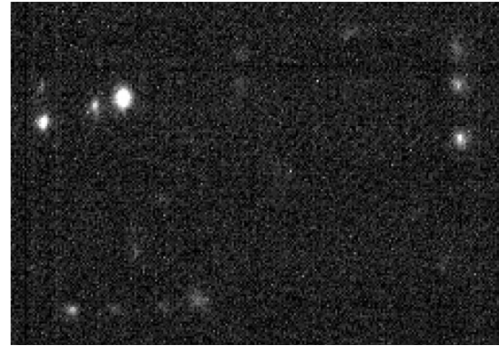
(b) Reverse bias electroluminescence image.
