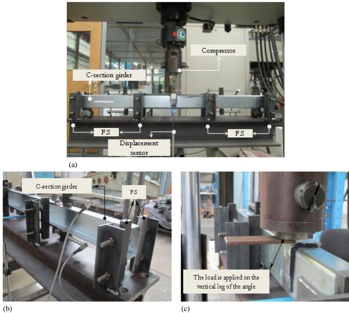
Figure 6.3: Test set-up (a) 3-points bending test (b) Fork supports used (c) Applying the load on the top edge of the vertical leg of the angle.
