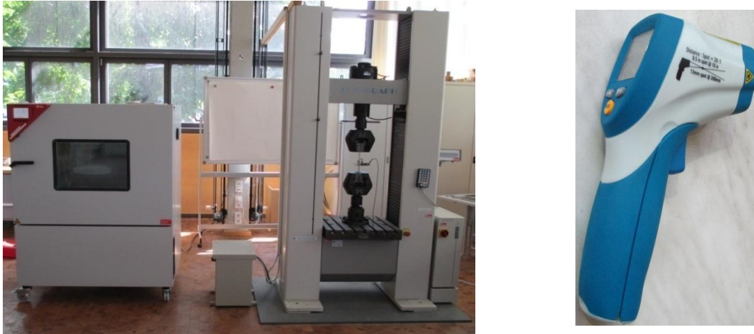
Figure 4.6: Test equipments Left: the climate chamber and the testing machine. Right: the laser thermometer used for measuring the temperature at the surface of the specimen
