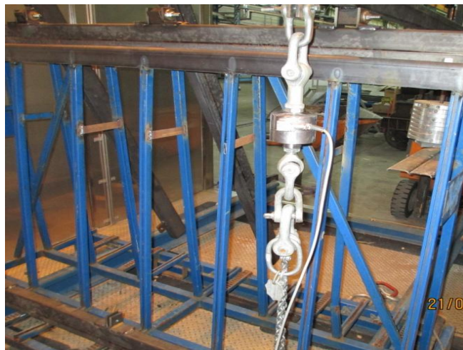
Figure 5.15: The creep machine and the calibration of the weights inside the climate chamber
