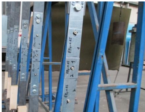
Figure 5.7: Long-term shear strain measurement
