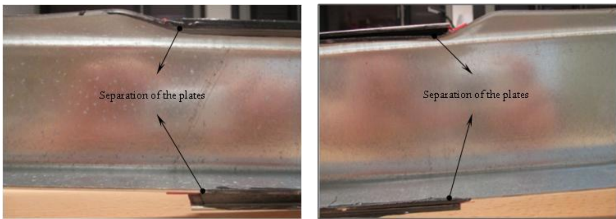
(b) The separation of the bonded plates in EP-U-B
