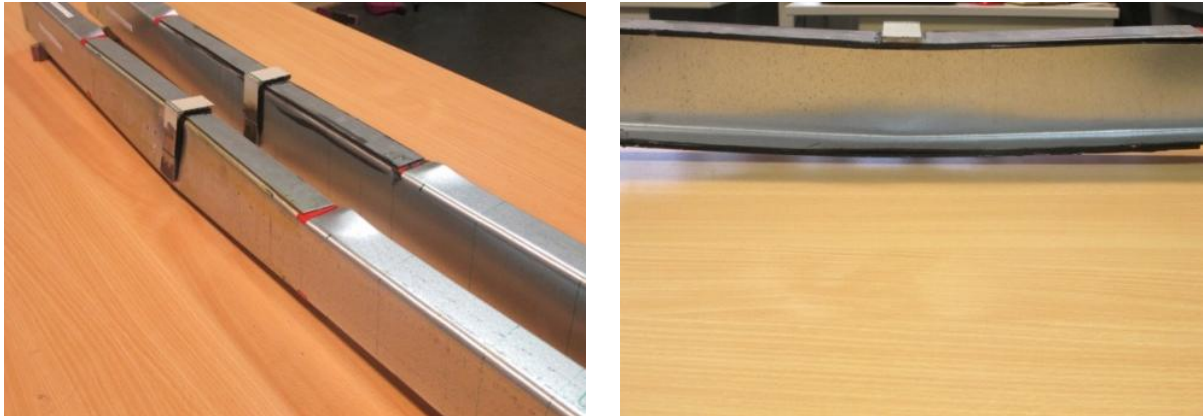
(a) Deformed girders of AC-U-B and EP-U-B (left) The curvature of the girders (right)
