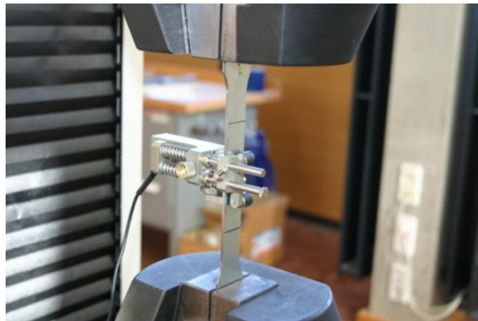
Figure 4.2: A tested specimen instrumented with a strain gage extensometer
