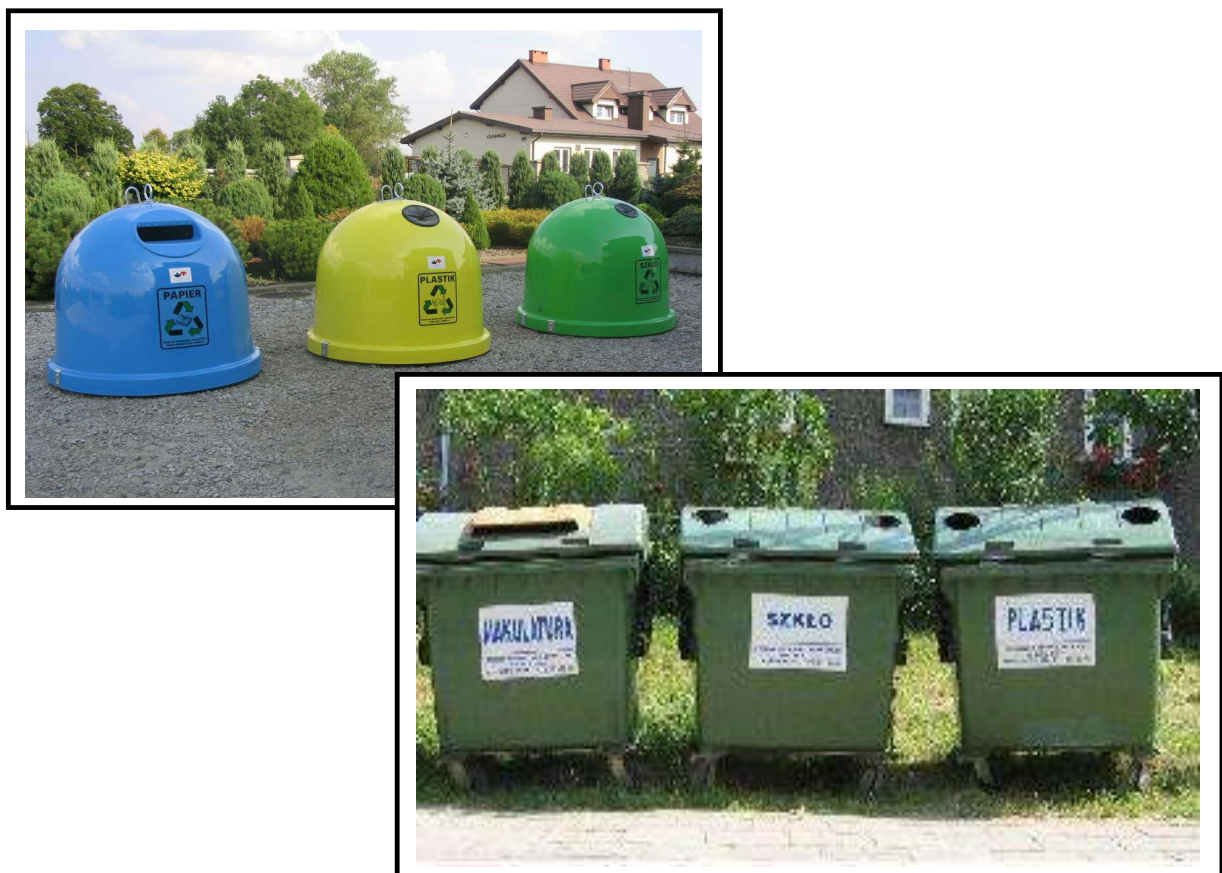
Figure II.2.5. Easy access ‘igloo’ and open-top containers for separate waste collection
