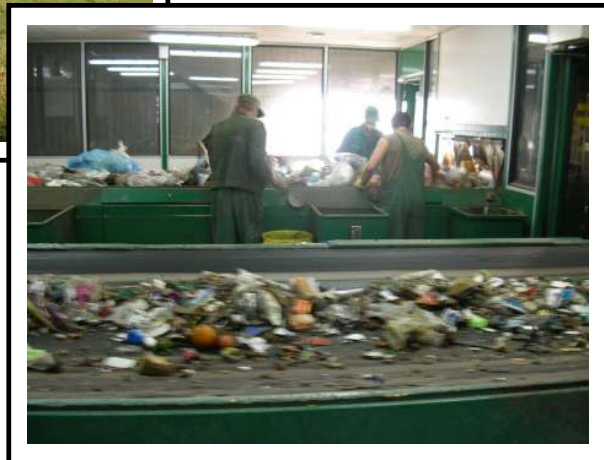
MWTF in Włocławek – manual belt sorting facility
