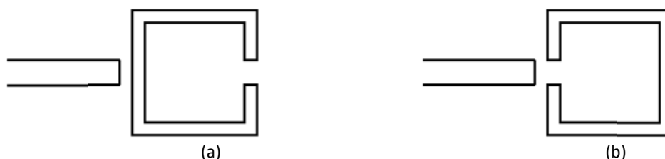
Figure 5-19: 2-ways of exciting square open loop resonator (a) Excitation of the resonator in a null of the fundamental mode (b) Excitation of the resonator symmetrically with respect to both open ends [50]
