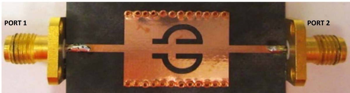
(a) 2-port complementary coupled resonator (CCR) fabricated using RT/Duroid 5880 substrate with a thickness of 0.508 mm and dielectric constant of 2.2 [103]
