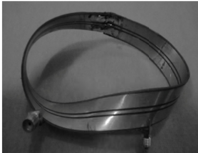
Figure 7-12: A prototype of CPW Möbius device with SMA connectors [19]
