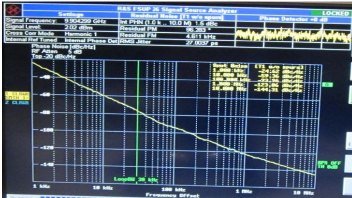
(a) Measured phase noise plot on R&S FSUP26 [102]
