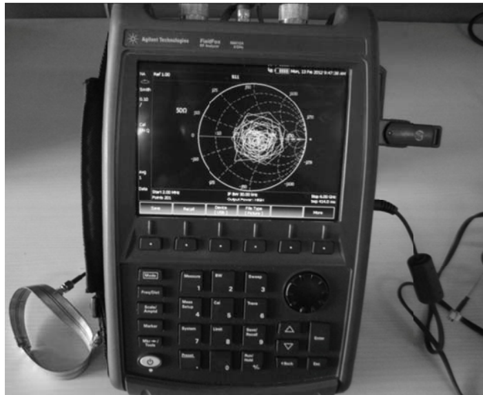
Figure 7-13: Agilent Analyzer N9912 with the device connected. The return loss test shows S_{11} parameter on Smith Chart from 2 MHz to 6 GHz. The display indicates the broadband coupling of signal into the device [19].
