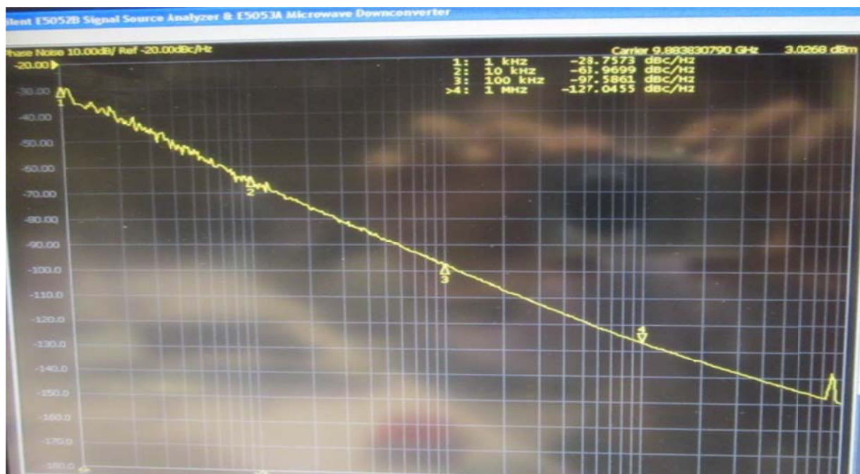
(b) Measured Phase noise plot on Agilent 5052B+5053A [102]
