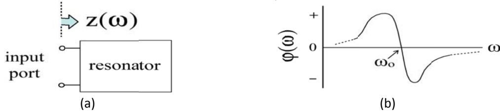
Figure 5-8: Examples of 1-port resonators (a) schematic of 1-port resonator (b) phase versus frequency response [22]
