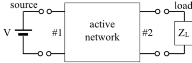
Figure 5-14: A typical 2-port oscillator model
