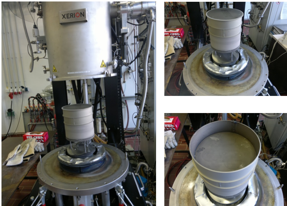
Figure 8 – Vacuum sinter furnace from Xerion.
