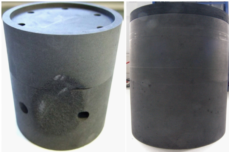
Figure 5.25.: Graphite susceptor a) attacked by NH_3 b) after microwave plasma enhanced experiment
