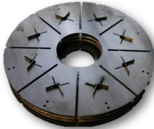
Figure 5.4.: Mo radiation shield
