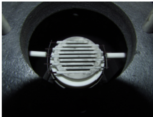
Figure 4.8.: DBD source mounted into the growth setup
