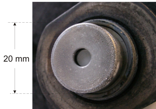
Figure 5.32.: Ga droplets on the seed-holder because of plasma instability
