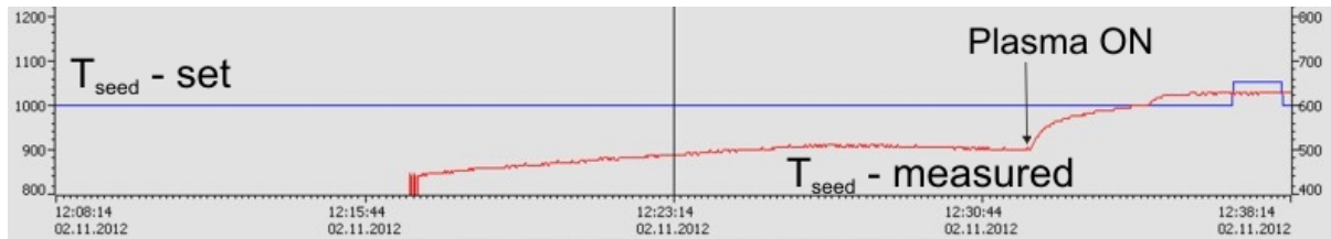
Figure 5.19.: T_{seed} vs t . Plasma ignited in the cavity
