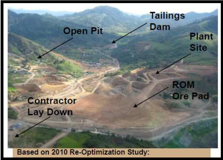
Figure 8: OGPI Conceptual Mining Arrangement (Source: OGPI Company profile November 2010)
