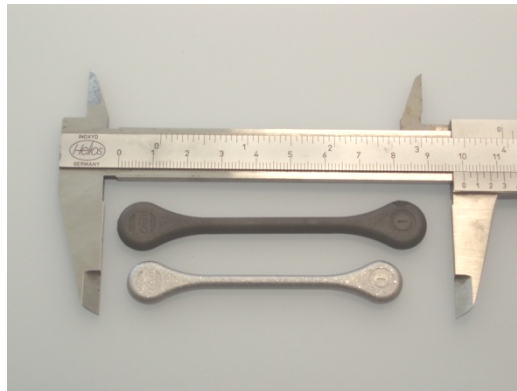
Fig. 3.2-2. Injection moulded and as-sintered “dog-bone” tensile test specimens. Top: The green sample; Bottom: The as-sintered sample
