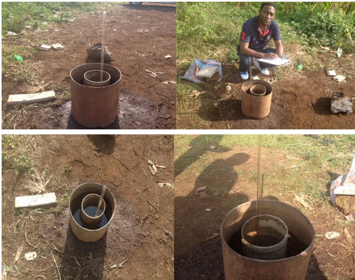
Figure 27: Double ring infiltration set-up during field test in Muea
