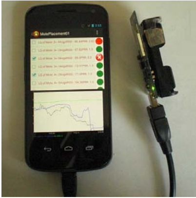
Fig. 1. Smartphone connected to a TelosB, gathering connectivity information; on the smartphone, link qualities are visualized through semaphores.
