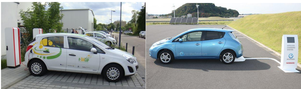
Figure 3.12: Electric vehicles being charged (a) based on cable and (b) based on wireless inductive charging [42]
