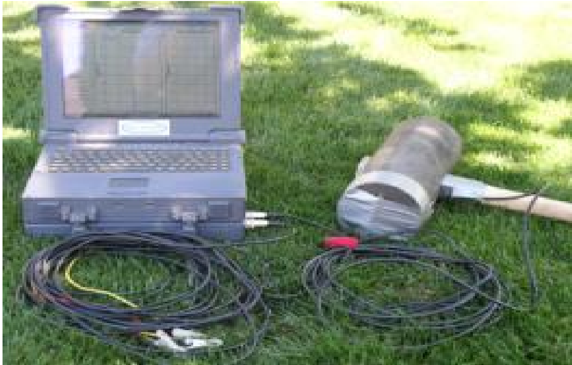
Figure 13: Picture of GF 2500 and hammer for data collection
