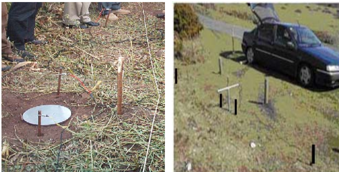
Figure 14: Illustration of data acquisition with hammer and plate method. (Groundflow, 2000)
