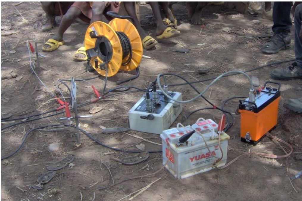
Figure 7: Arrangement for data acquisition in Lund 2-D multi-electrode resistivity survey.
