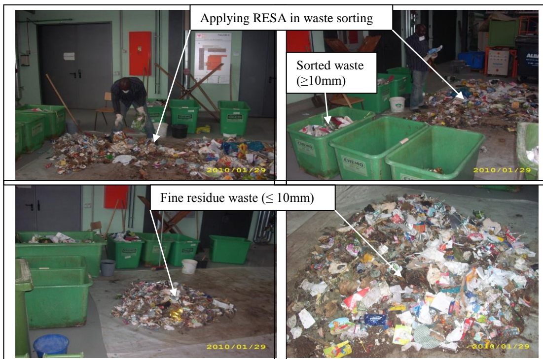
Figure 4.5 Application of RESA in sorting commingled waste
