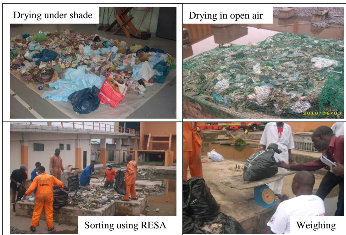
Figure 4.3 Waste pretreatment and sorting for plastic recovery
