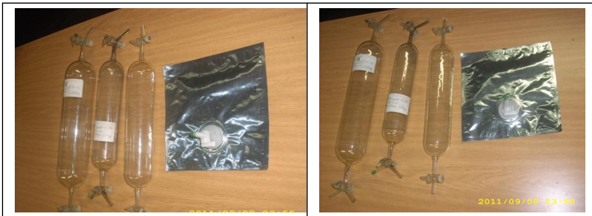
Figure 10.1 Gas jars and gas bag used for collecting exhaust and pyrolysis gases
