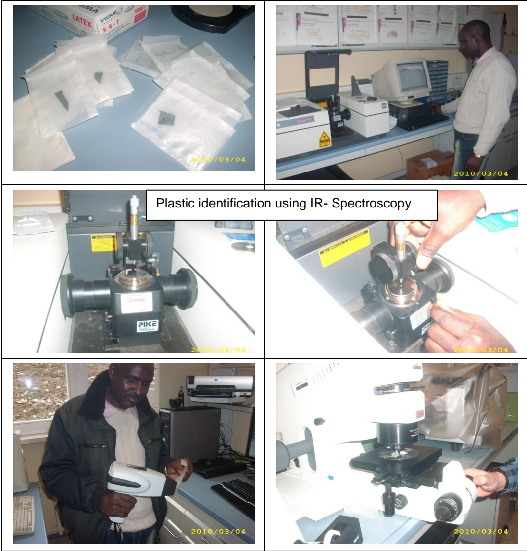
Q: Plastic waste identification using near IR spectroscopy
