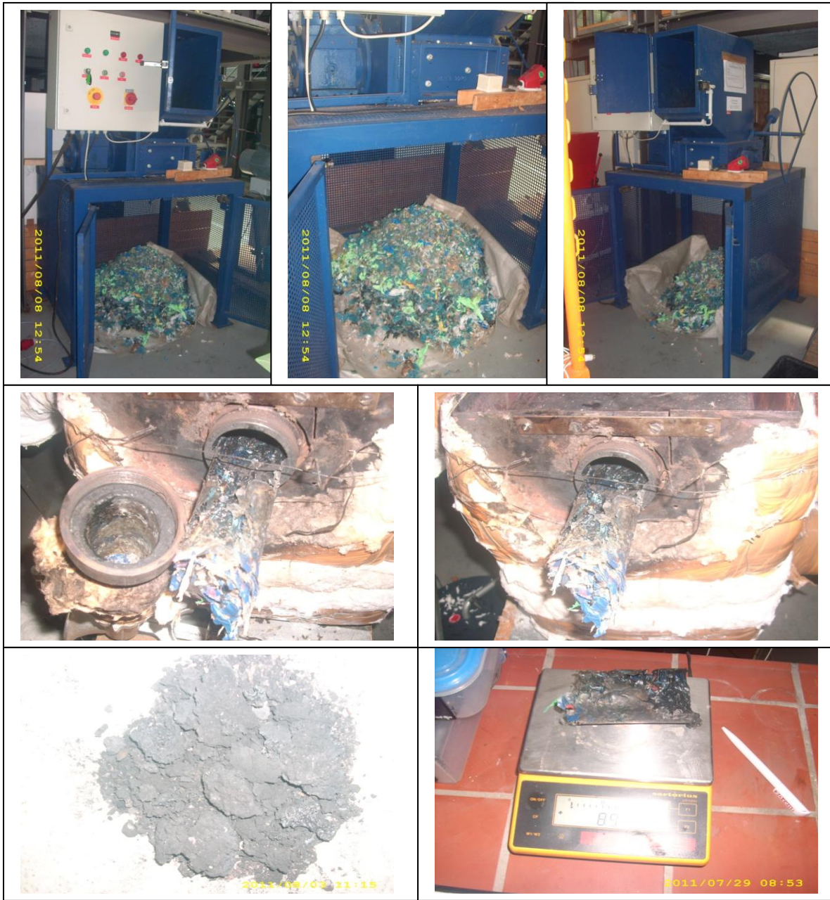
T: Pretreatment and use of plastics for energy recovery
