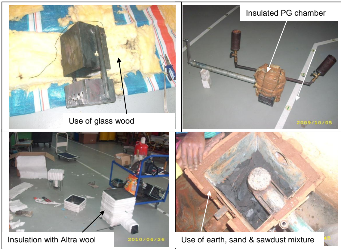
Figure 8.18 Insulation of PG chamber and external casing
