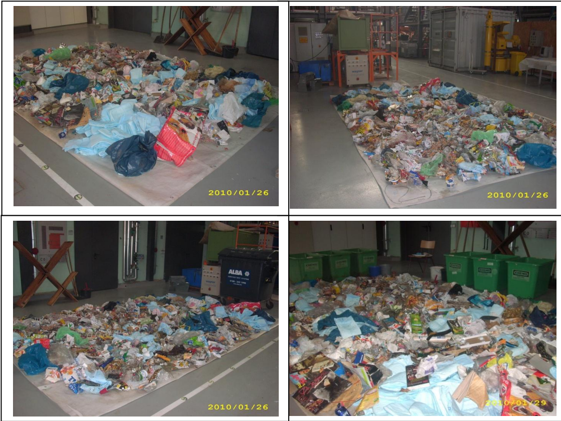
I: Waste drying before sorting to remove moisture
