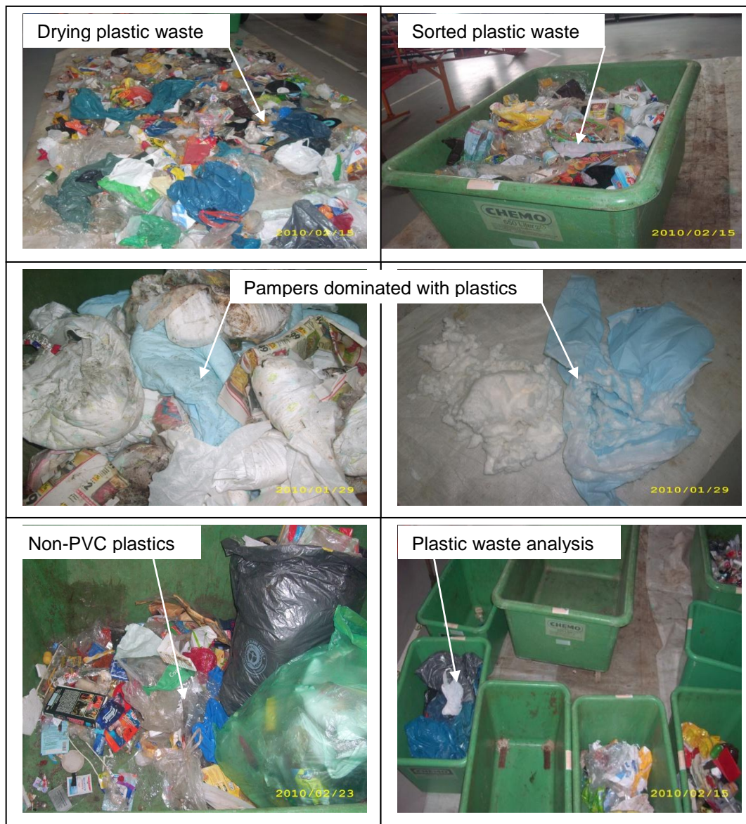
Figure 4.8 Plastic waste fraction pretreatment and sorting
