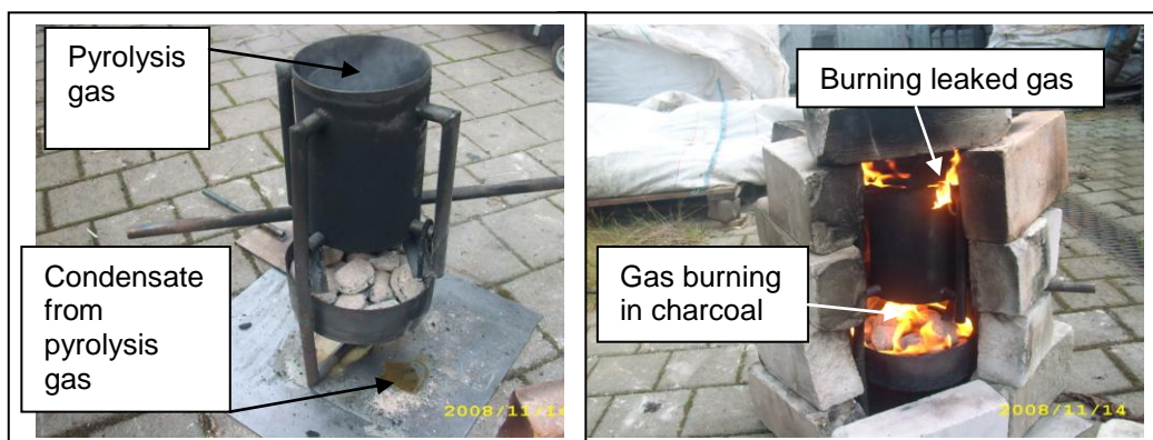
Figure 8.13 Pyrolysis gas flows to combustion chamber and burns in-situ
