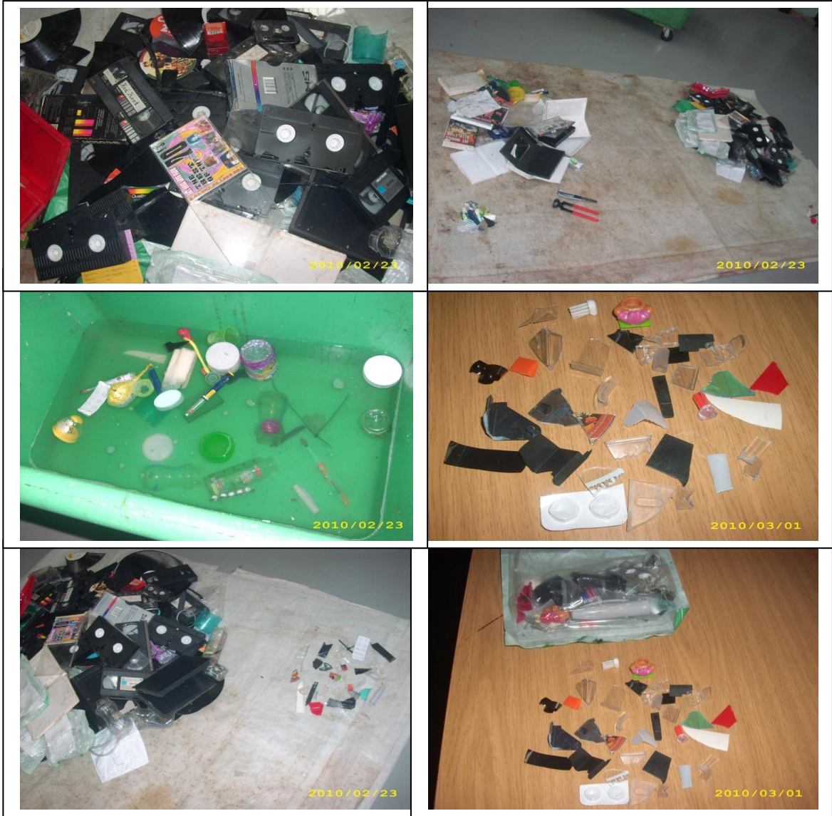
P: Plastic waste identification using sink-float test
