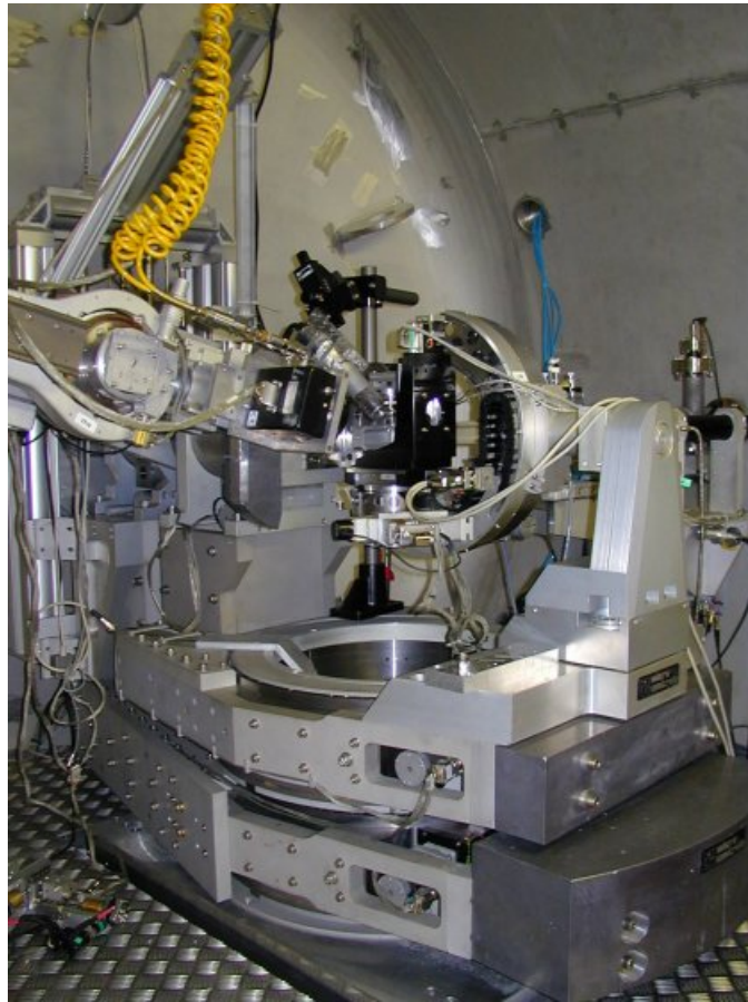
Figure 3.4: 2+4-circle diffractometer + 2 circle analyser stage at ID01 (ESRF) [105].
