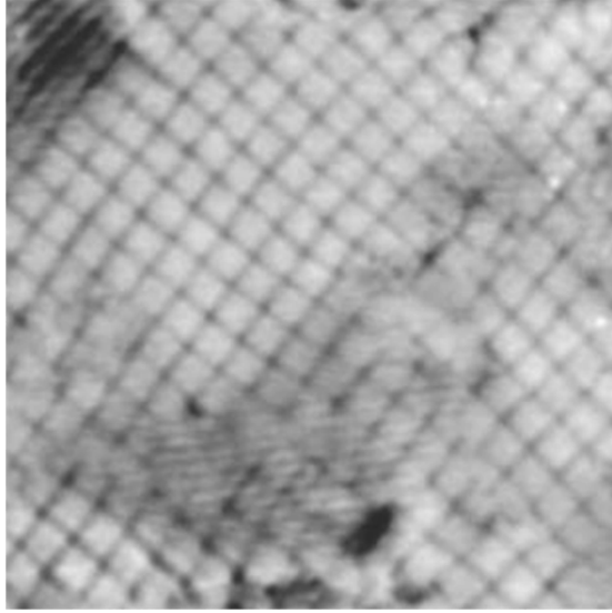
Figure 2.13: Plane view TEM micrograph of 20-nm-thick Ge/Si(001) with the cross hatch pattern [90].
