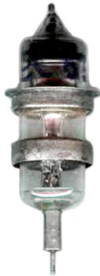
Figure 3- The light-house tube EC 55 [4]-[6]
