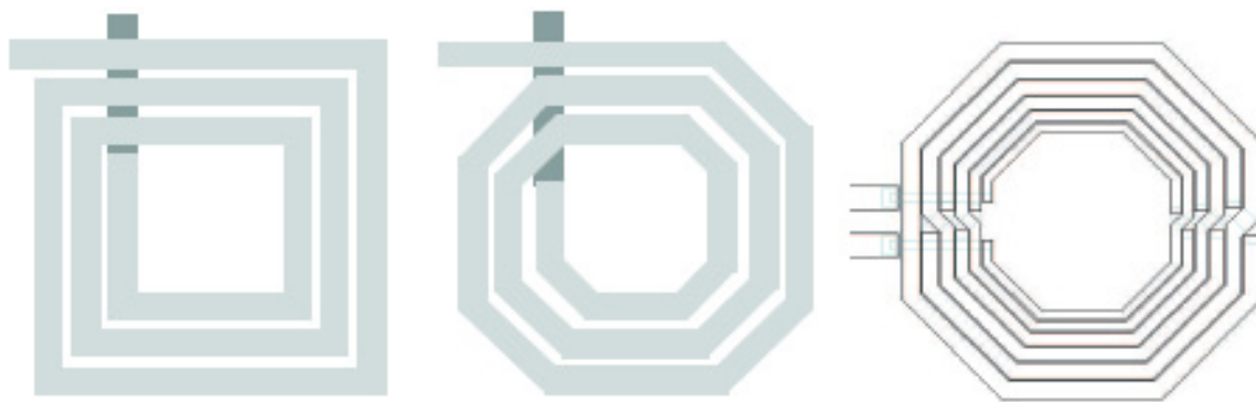
Figure 3-17 Quadrilaterals, octagonal and symmetrical octagonal inductor designs.
