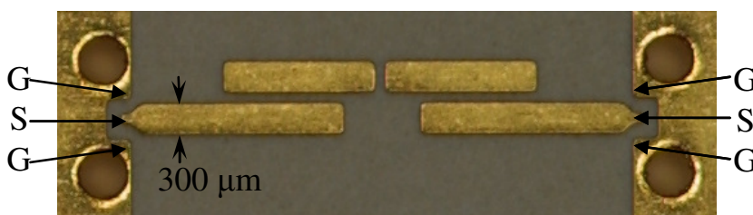
Figure 4. 43 On-board filter photo with marked probing positions.
