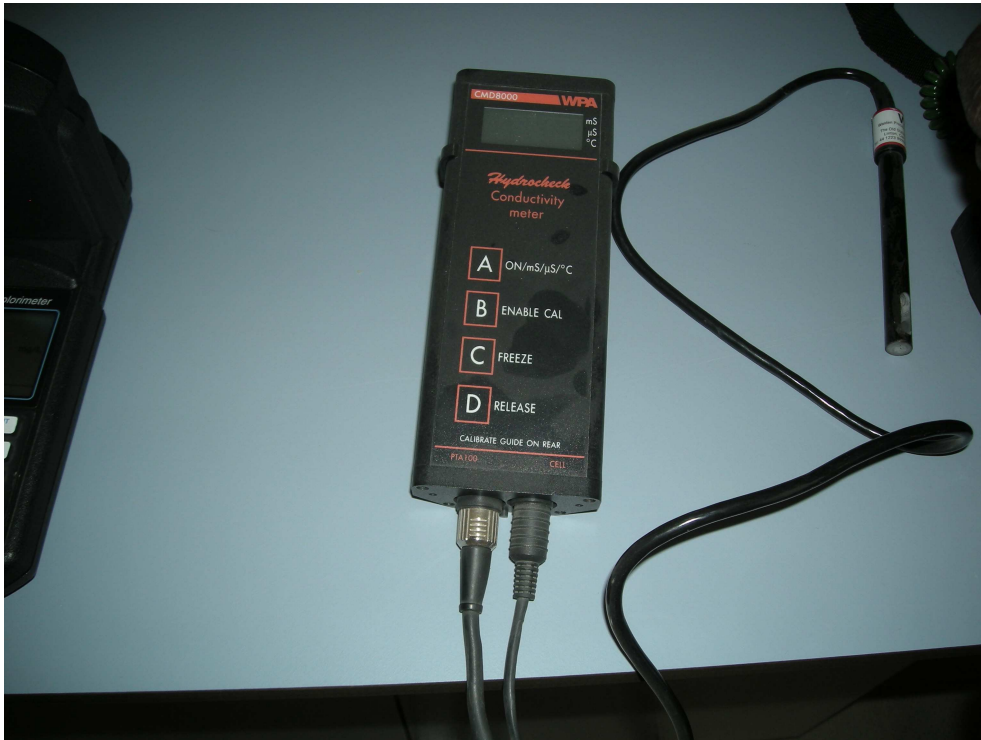
Figure 3.11 Electrical Conductivity Meter from Gombe Regional Laboratory
