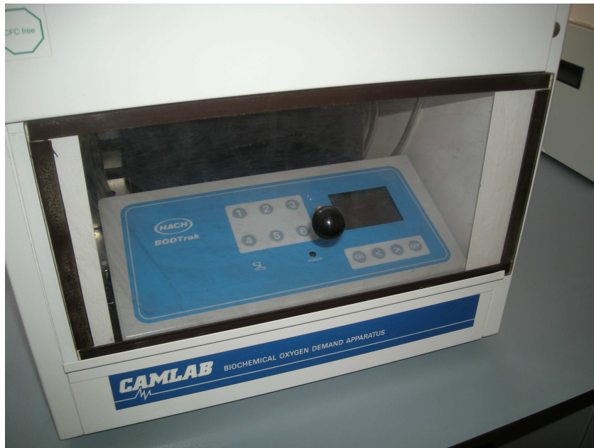
Figure 3.14 Biochemical Oxygen Demand (BOD) Reactors from Gombe Regional Laboratory
