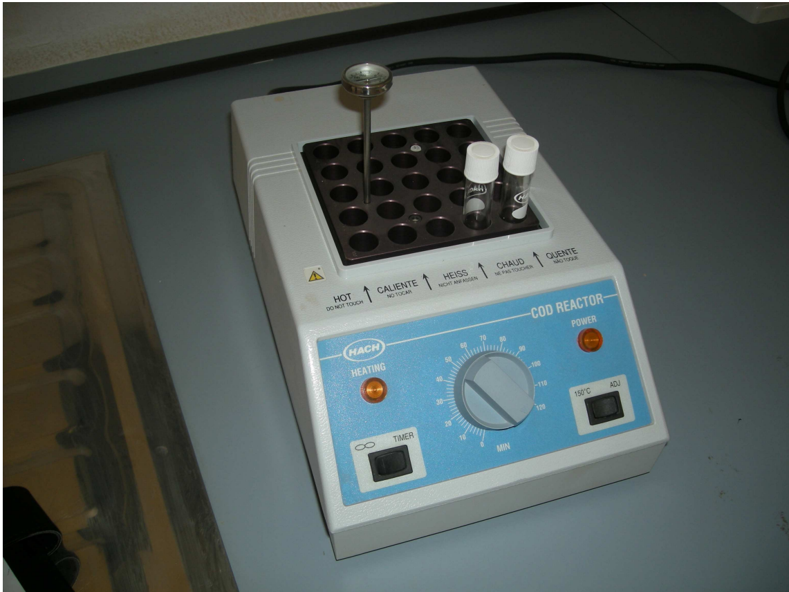
Figure 3.13 Chemical Oxygen Reactors from Gombe Regional Laboratory
