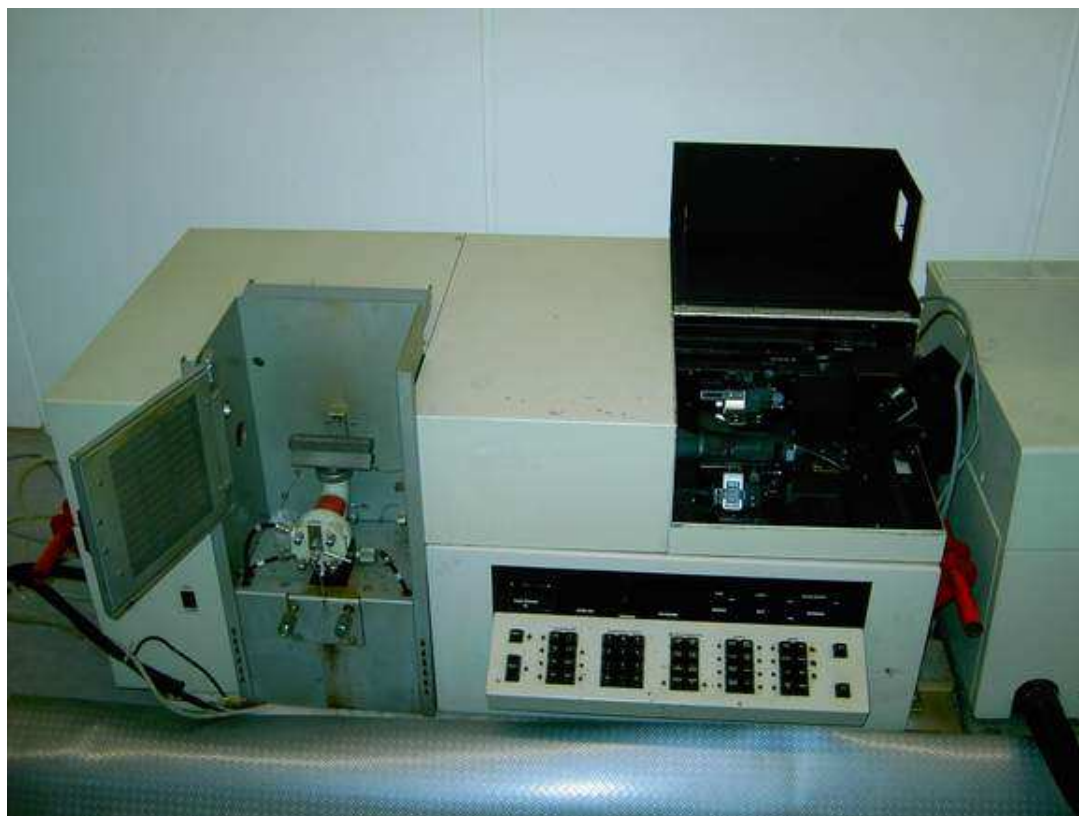
Figure 2.8 Perkin Elmer AAS 5000. With Auto Sampler AS 70. Programmer AS 40. Zeeman HGA 500. Programmer HGA 500. Analysis Unit Shimadzu Chromatopac C-R6A.
