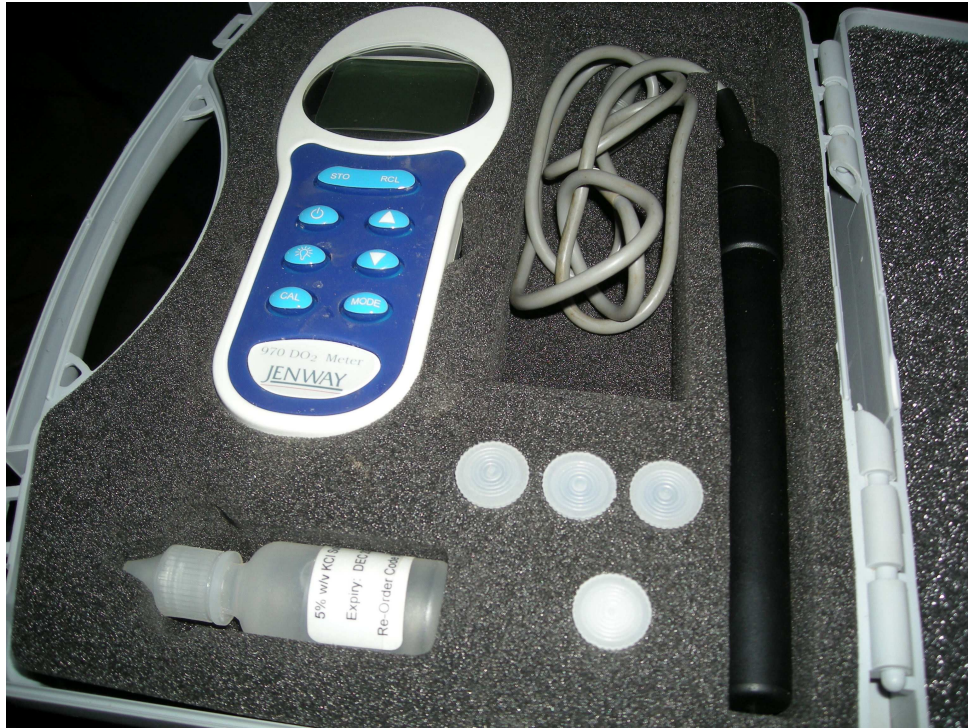
Figure 3.3 Dissolved Oxygen (DO) Meter) from NNPC Kaduna
