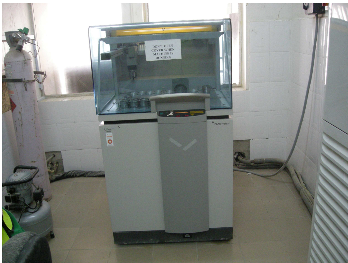
Figure 3.9 X-Ray Fluorescence (XRF) Spectroscopy from Ashaka Cement Factory
