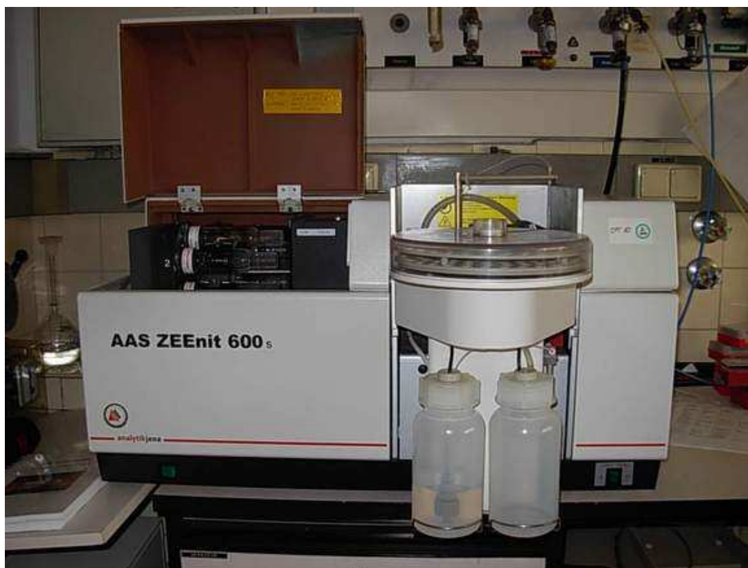
Figure 2.9 AAS ZeeNit 600 with Graphite Tube Control (Source; Analytik Jena)
