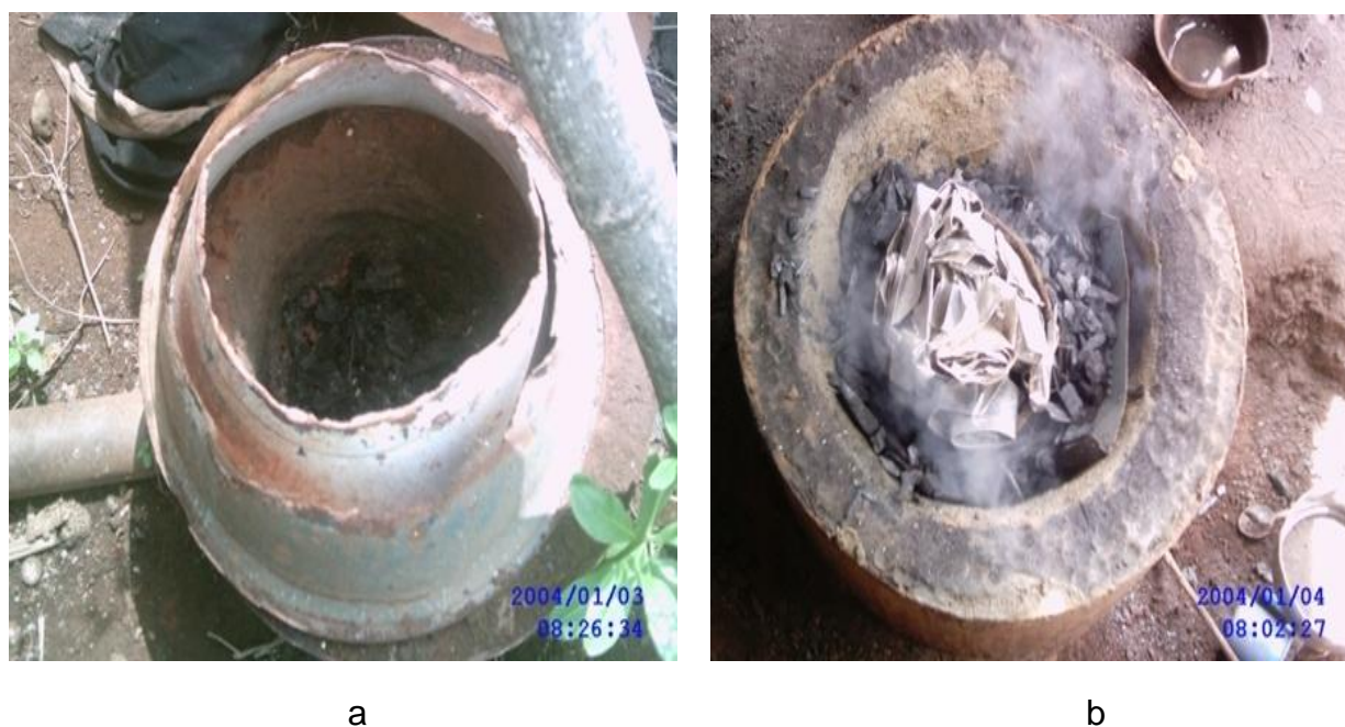
Figure 17 Heating chamber constituting a cylindrical metal device into which charcoal or wood is used for energy generation. Note in a) ventilation pipe on surface and b) ventilation pipe buried. (Source: author's fieldwork)
