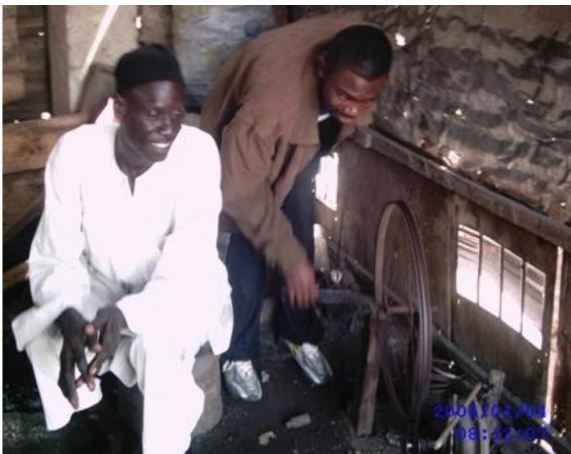
Figure 16 Air ventilation unit components of local macocot pot production plant in Cameroon. (Notice chord fixed both round the wheel and motor in front of wheel) Source: author's fieldwork.
