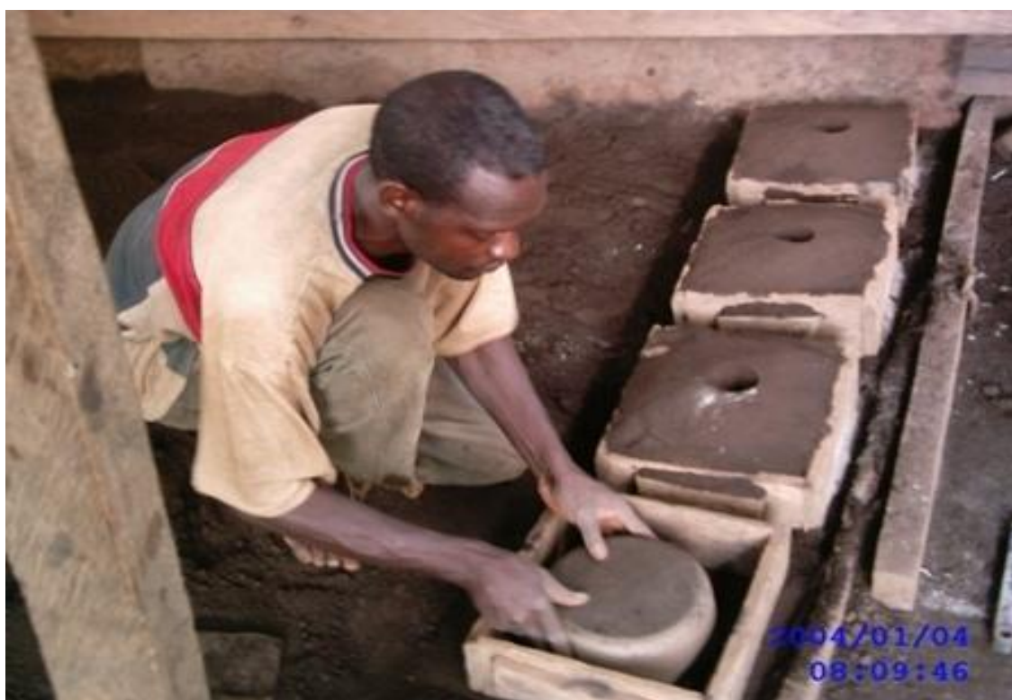
Figure 18 Construction of molds for production of household cooking pots (Source: author's fieldwork)
