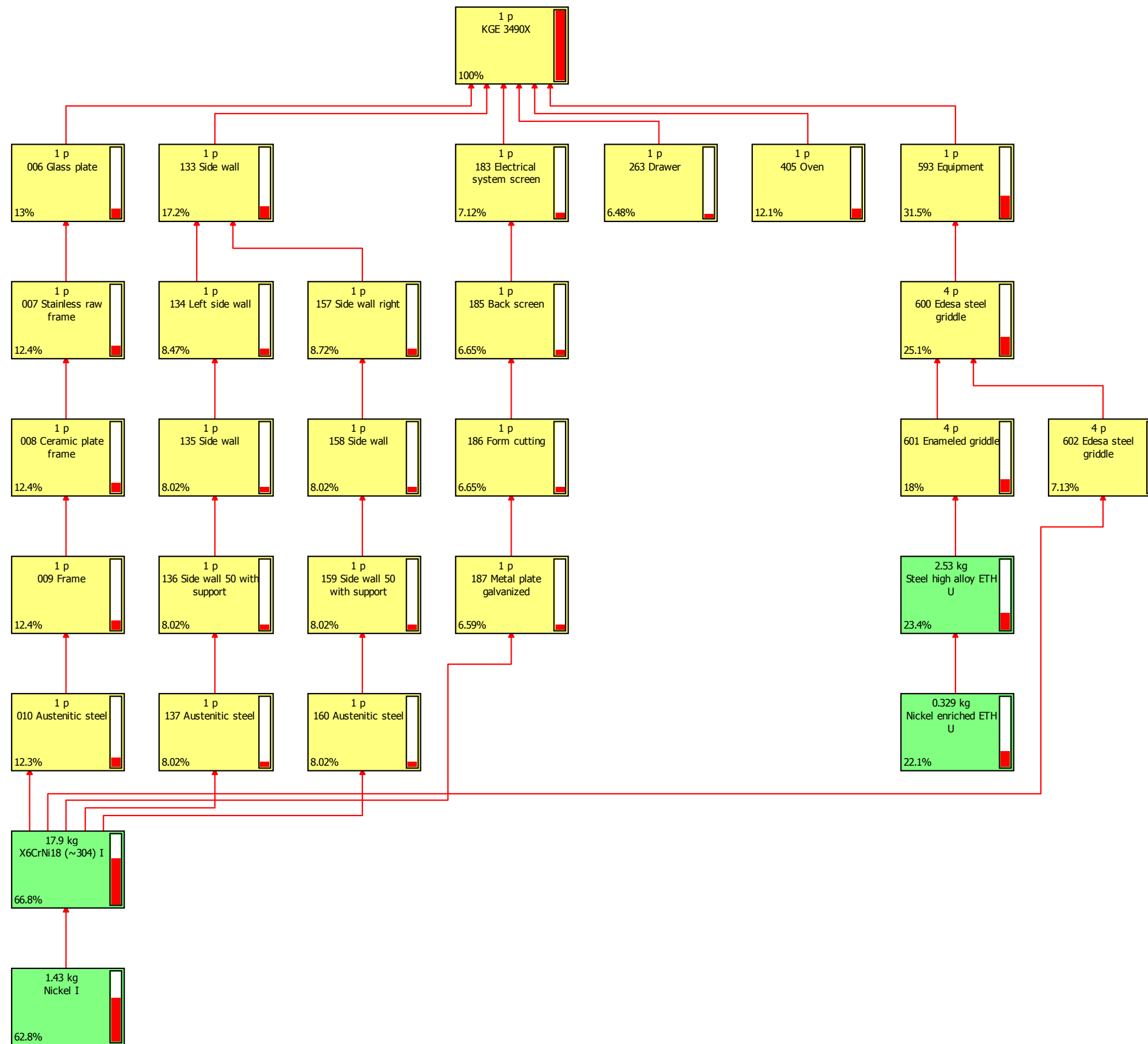
Figure 4 Normalization, CML 2 2000, with respect to acidification, cooker without EoL and without use phase. Units: percentage, 6% cut-off.
