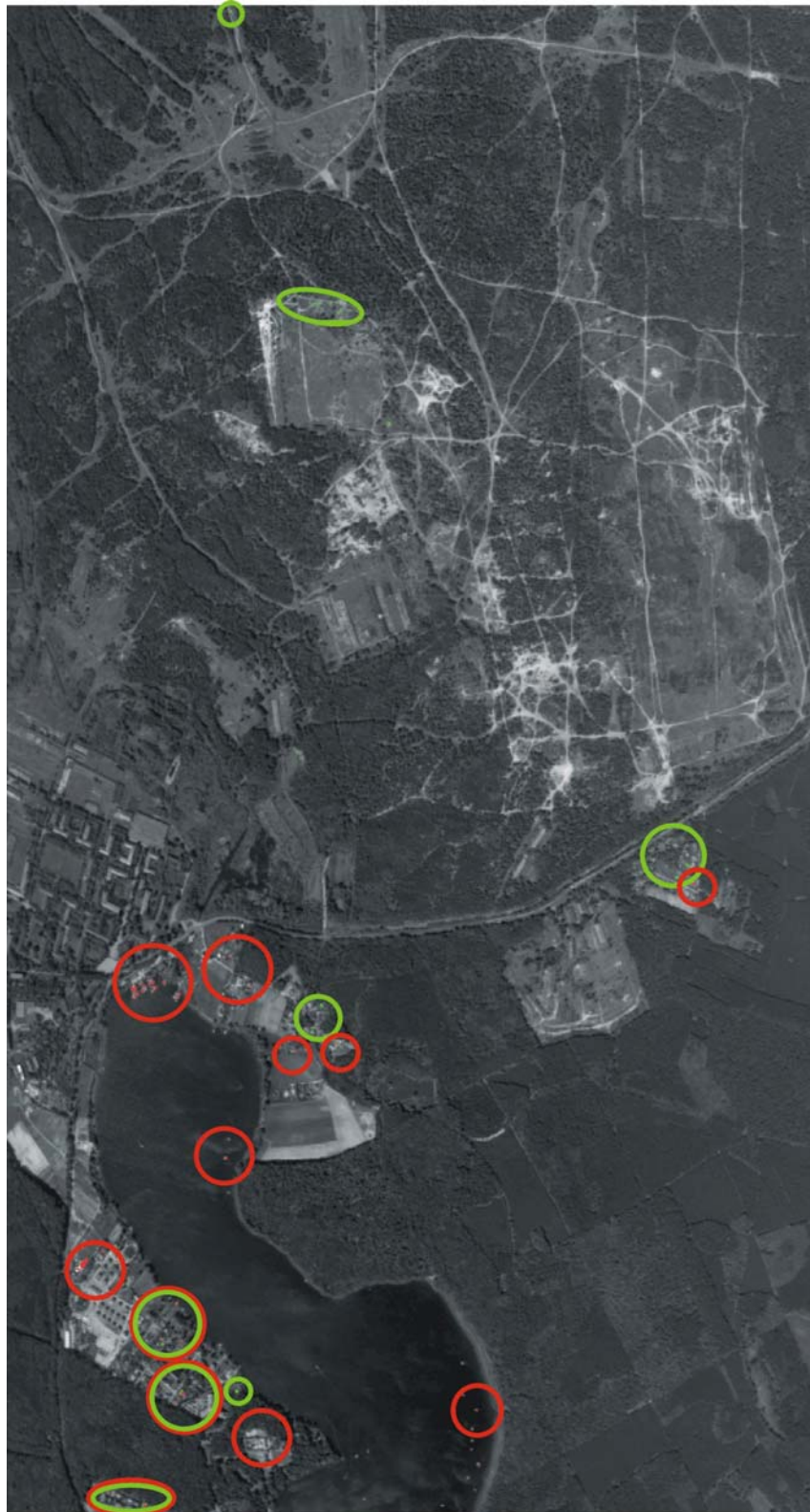
Figure 7-3: Hydrocarbon abundances (mainly plastics and wood) detected in the HyMap dataset of the former military training area Döberitzer Heide from 1999 and separated in two groups: aliphatics (green pixels, circled green) and aromatics (red pixels, circled red). Summation of three band differences calculated each for the region 1,669 nm–1,694 nm and 1,706 nm–1,730 nm, minimum threshold absorption feature depth (band difference) of 0.04 (4 % reflectance).
