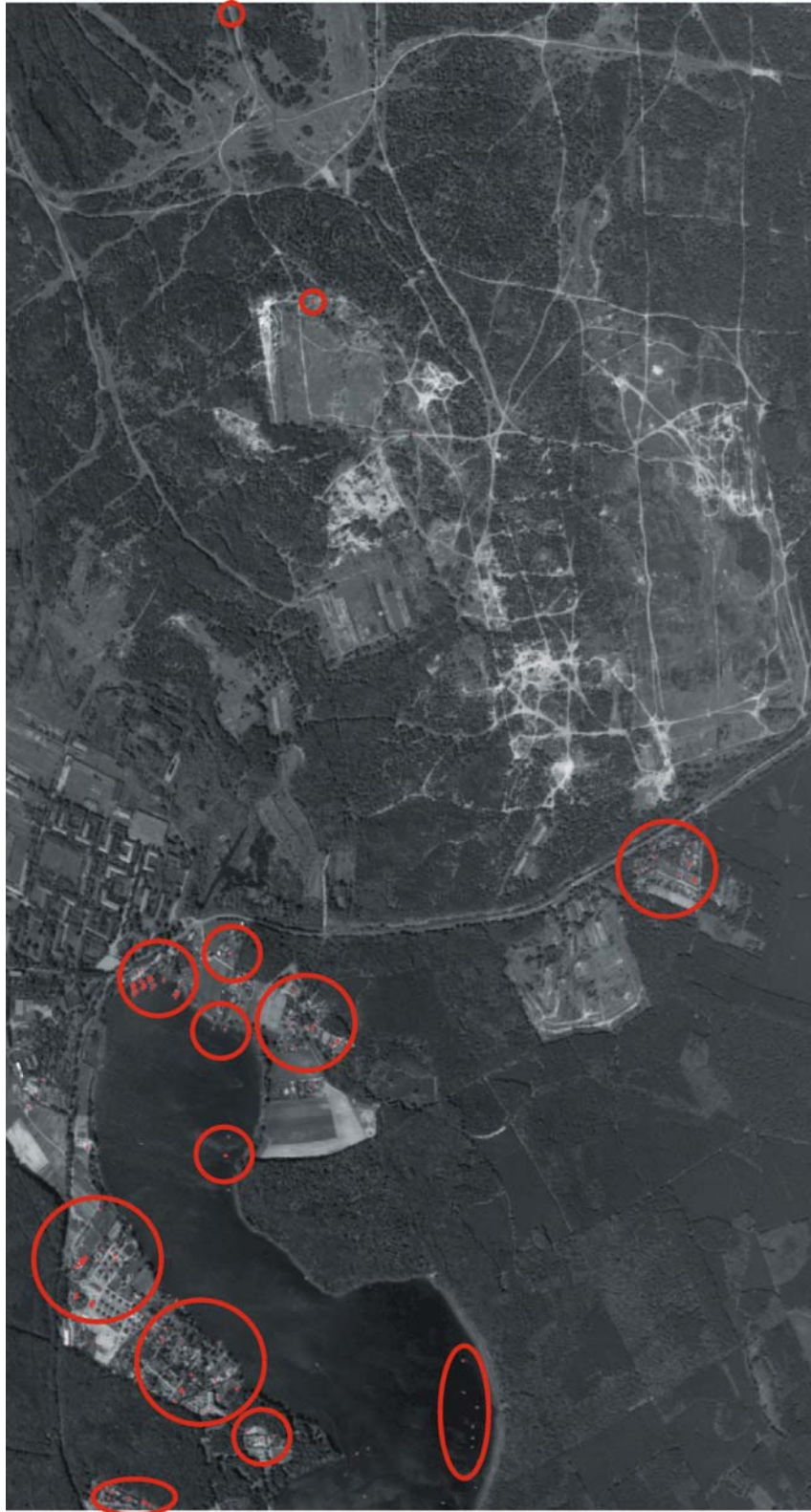
Figure 7-2: Hydrocarbon abundances (mainly plastics and wood) detected in the HyMap dataset of the former military training area Döberitzer Heide from 1999. Hydrocarbon abundances are pixels marked red and circled for better visibility. Summation of six band differences calculated for the region 1,669 nm – 1,730 nm, with a minimum threshold absorption feature depth (band difference) of 0.08 (8 % reflectance).
