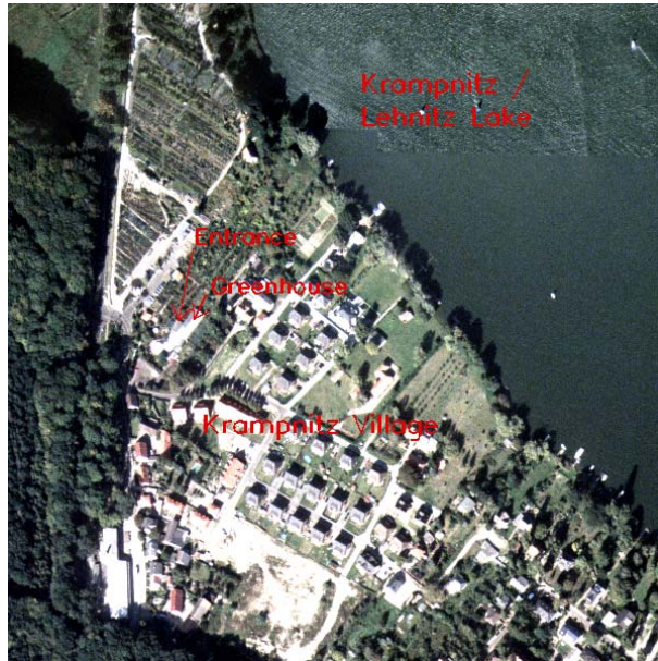
Figure 7-4: Color aerial image (RGB) acquired in 2000, Krampnitz village, resolution 0.5 m. The greenhouse and entrance, detected as aromatic and aliphatic plastic respectively, are noted.
