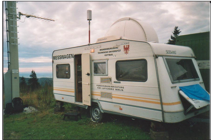
Fig. 2.8.a. For the FELDEX 2000-campaign near Frankfurt the CRDS-set-up was installed in a caravan. The gas inlet can be seen on the top, the pump was deposited in the boot on the right.
