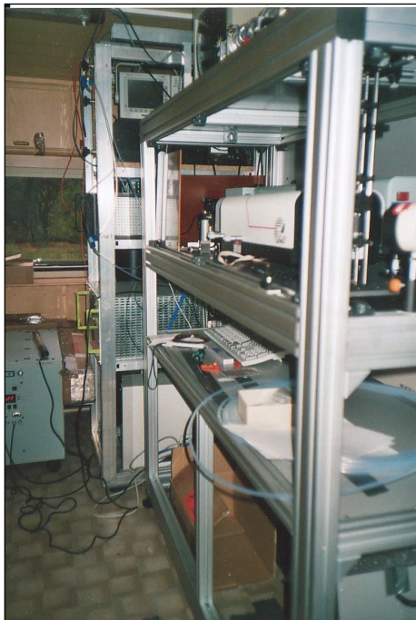
Fig. 2.8.b. Rack containing the set-up including pump laser, OPO and measurement cell. In the rear the laser power supply (left) and the rack with the gas mixing system can be distinguished (right).
