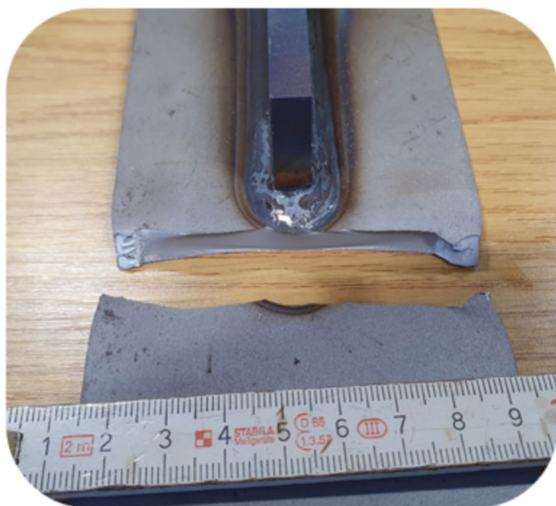
Fig. 9 Specimen with LTT single weld pass after fatigue testing. The crack propagated along the weld toe
