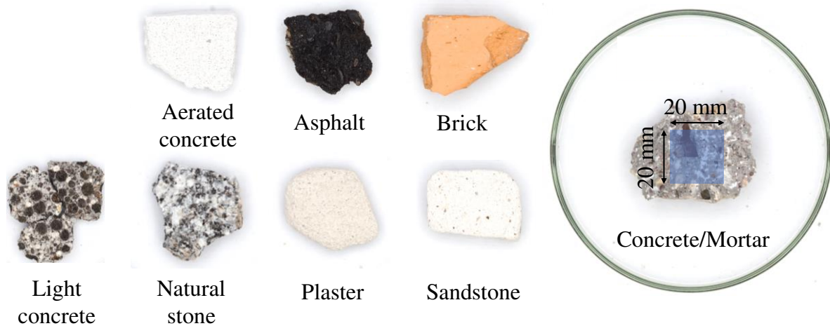
Figure 1: Exemplary pictures for each material group and the measuring area of LIBS on a concrete sample (blue square).
