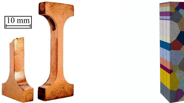
Fig. 2. (a) miniature creep specimens; (b) 3D FE model of the grain structure in the gauge length.
