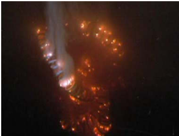
Picture 1 Plasma generated on the metal coil as substrate for electro-deposition application of metal
