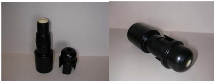
Picture 4: Sample holder for holding the lens curvatures in front of the capillary discharge site
